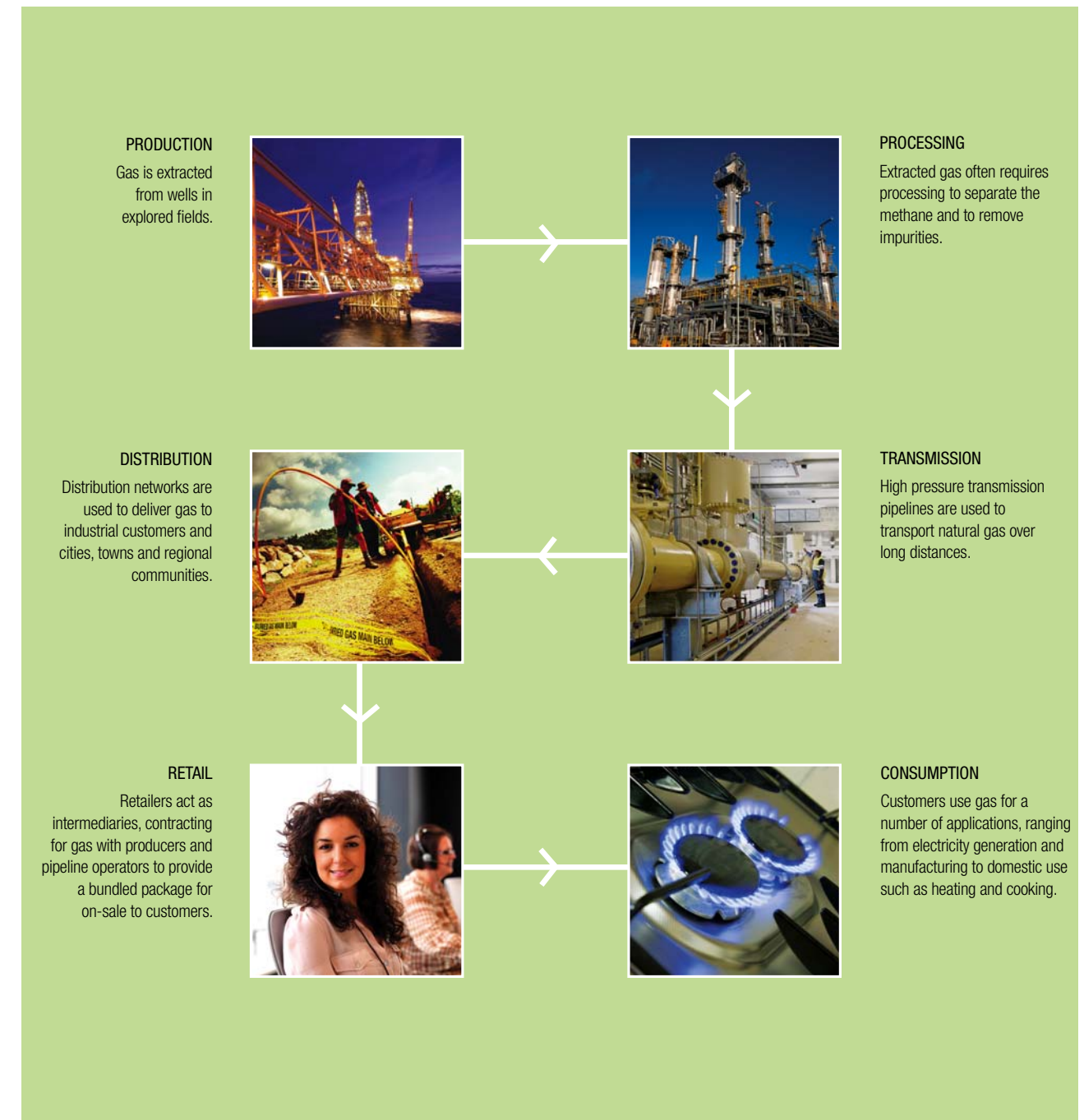
Figure 3.1 Domestic gas supply chain
