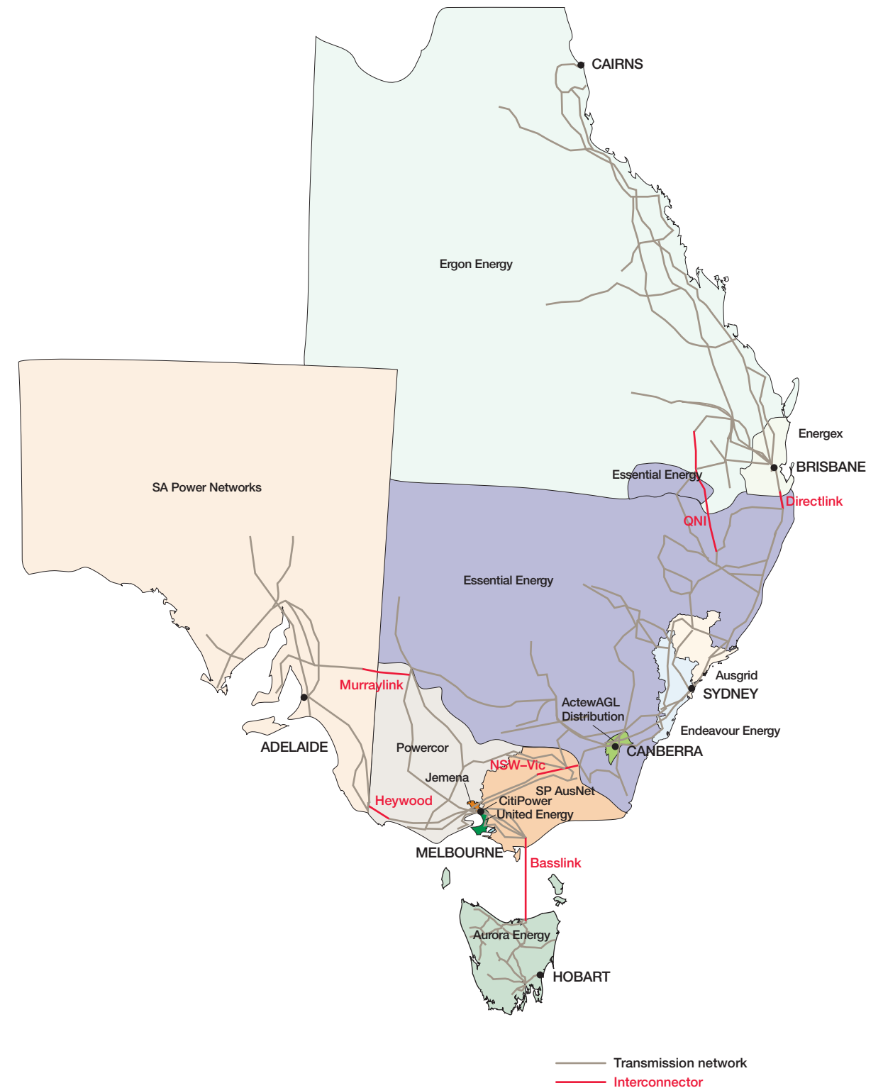
Figure 2.1 Electricity networks in the National Electricity Market
