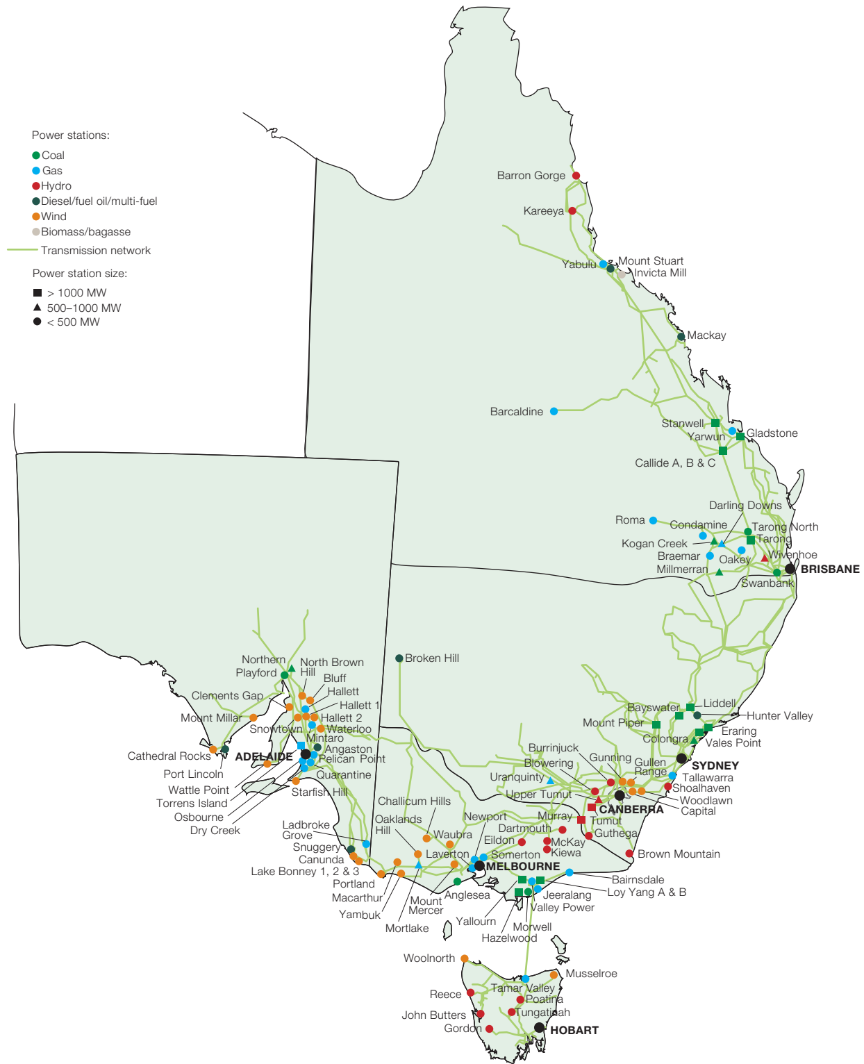
Figure 1.4 Electricity generation in the National Electricity Market
