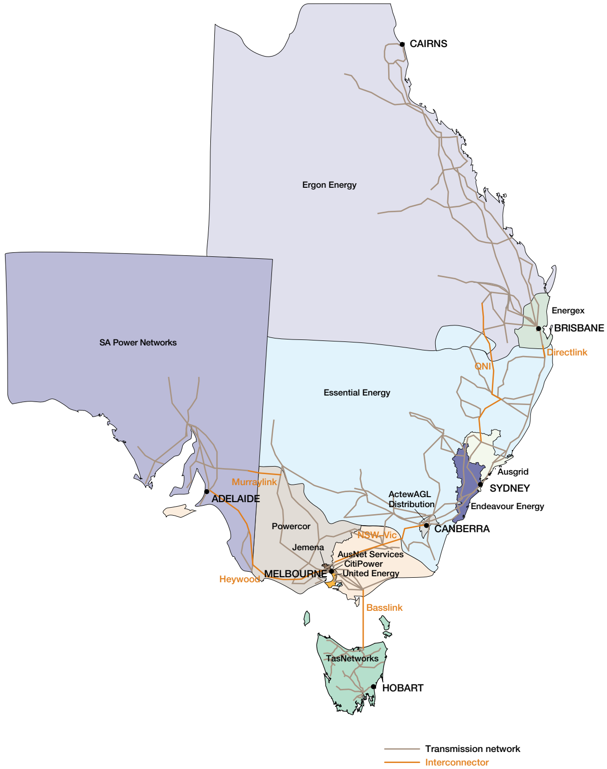
Figure 2.1 Transmission grid and distribution networks in the National Electricity Market
