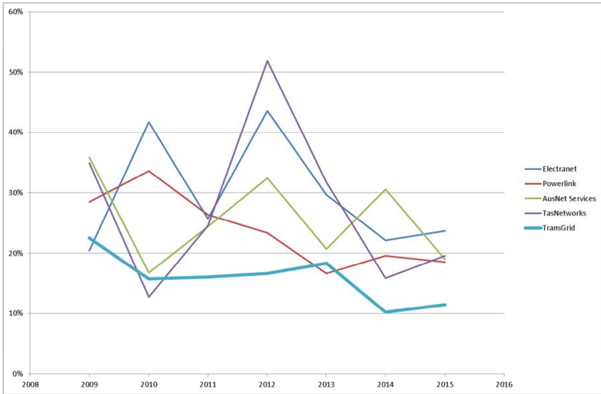
Figure 16.1: Fault outage rates – transmission lines
