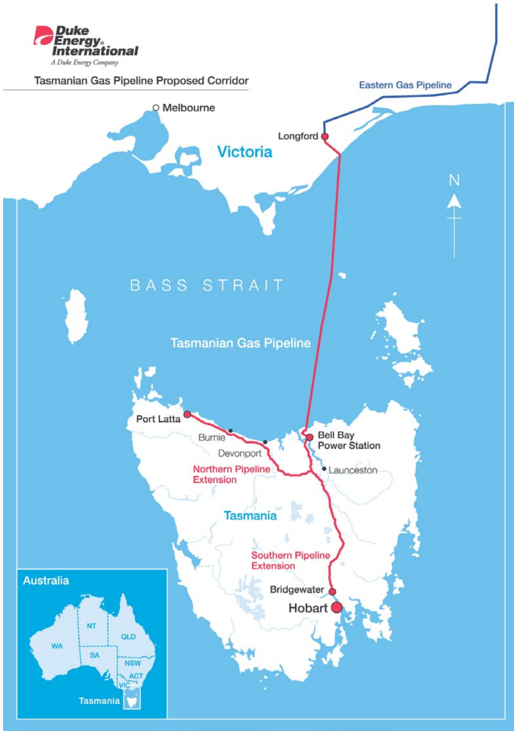
Figure I.10: The Tasmanian natural gas pipeline
