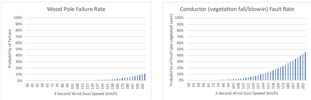
Figure A2: Vulnerability curves for pole failure and conductor faults
