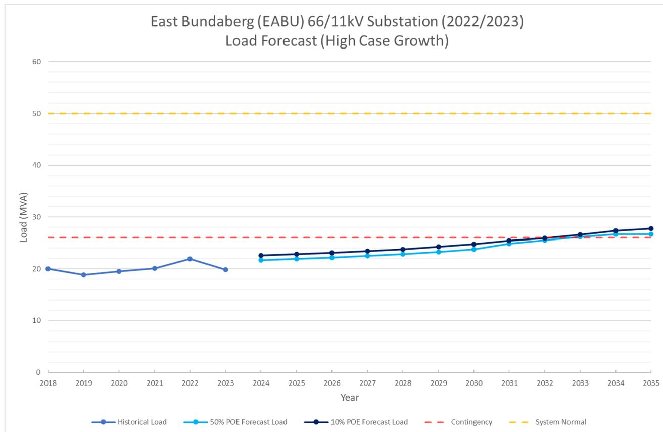
**Figure 22: East Bundaberg Substation high growth load forecast**
