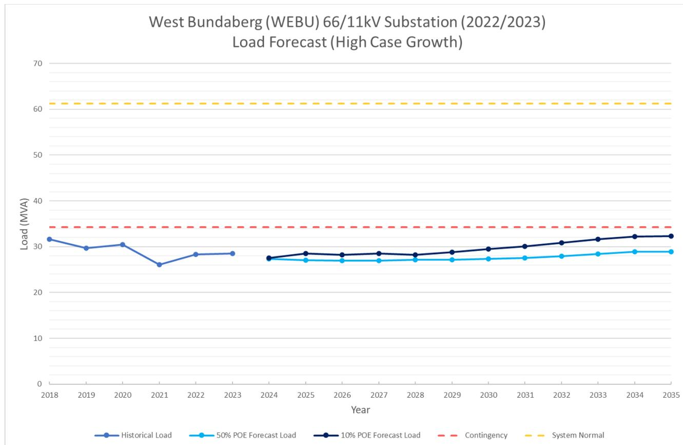
**Figure 20: West Bundaberg Substation high growth load forecast**
