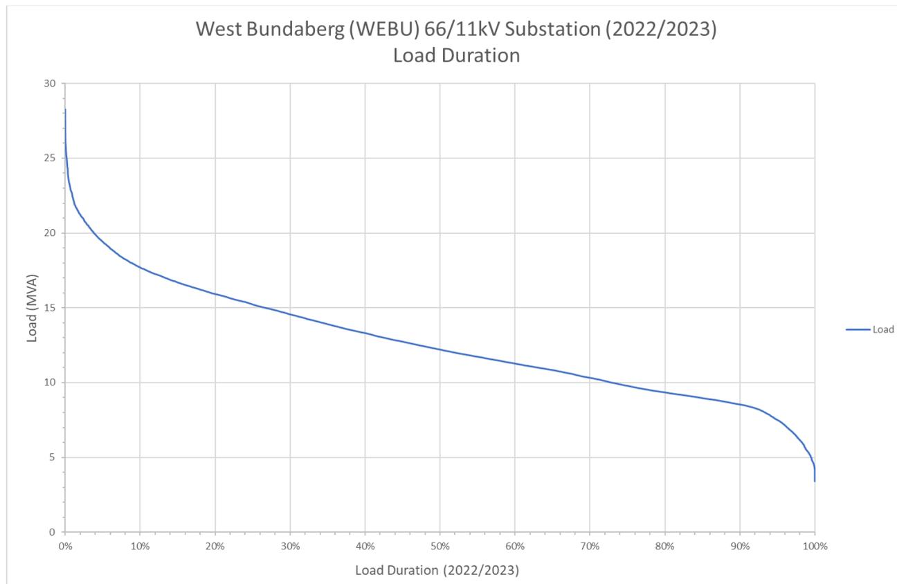
**Figure 8: West Bundaberg Substation load duration curve**
