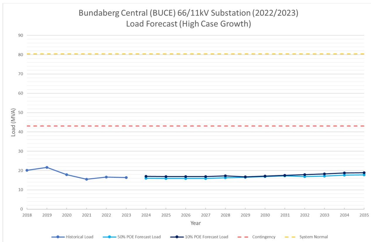
**Figure 21: Bundaberg Central Substation high growth load forecast**
