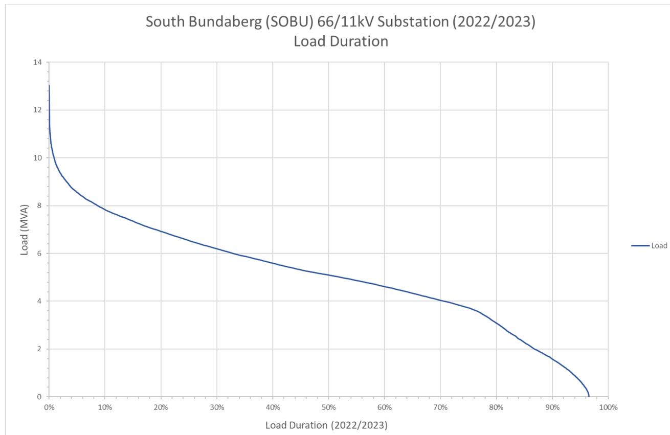
**Figure 11: South Bundaberg Substation load duration curve**
