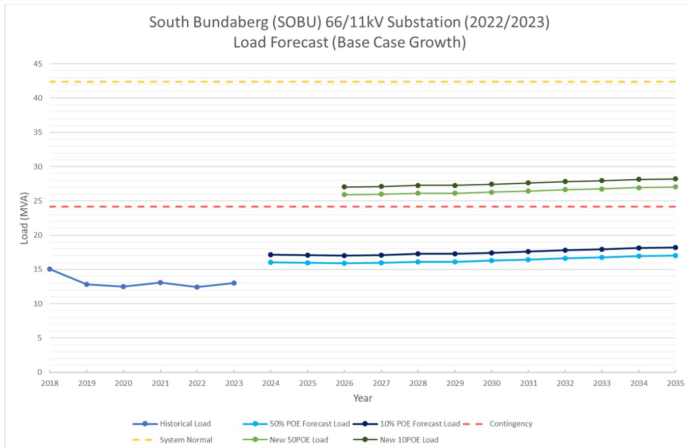
**Figure 19: South Bundaberg Substation base case load forecast**
