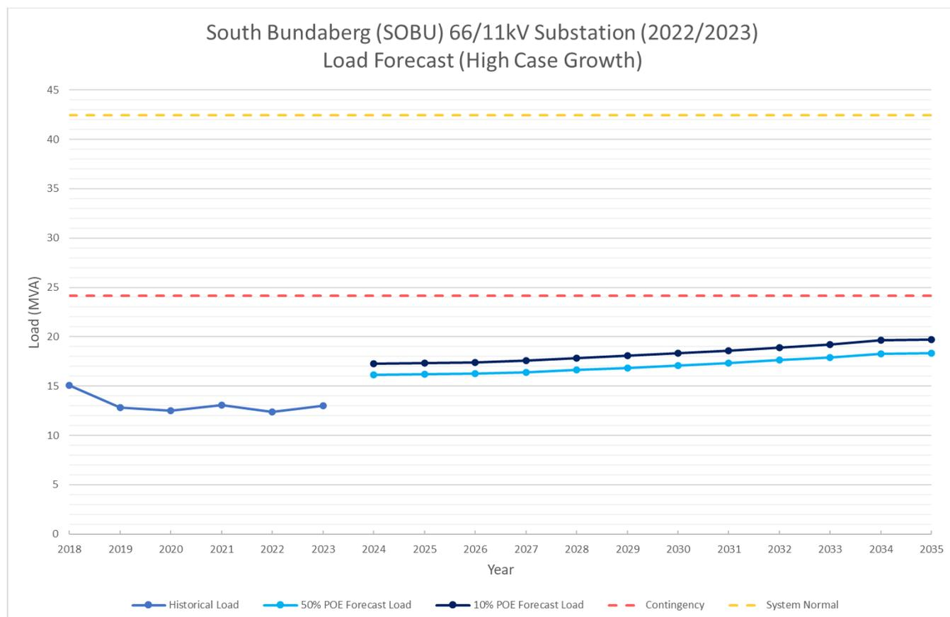
**Figure 23: South Bundaberg Substation high growth load forecast**
