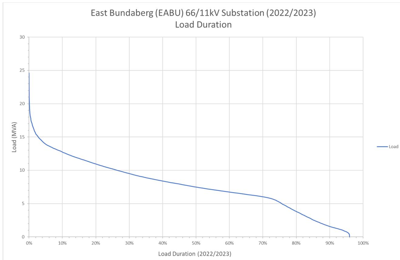
**Figure 10: East Bundaberg Substation load duration curve**
