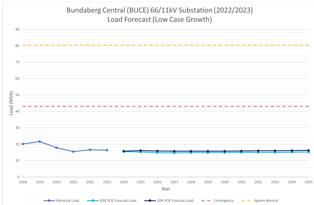
**Figure 25: Bundaberg Central Substation low growth load forecast**
