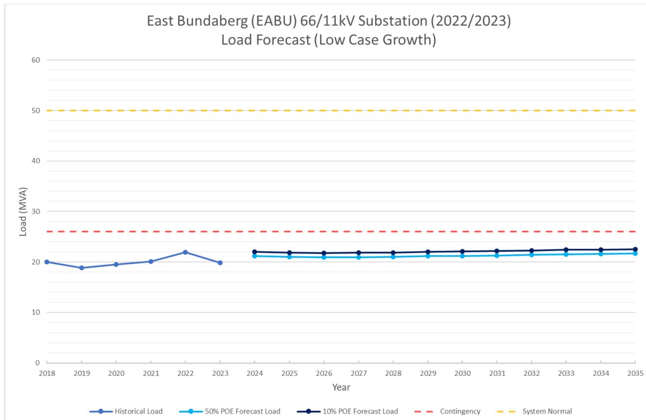
**Figure 26: East Bundaberg Substation low growth load forecast**
