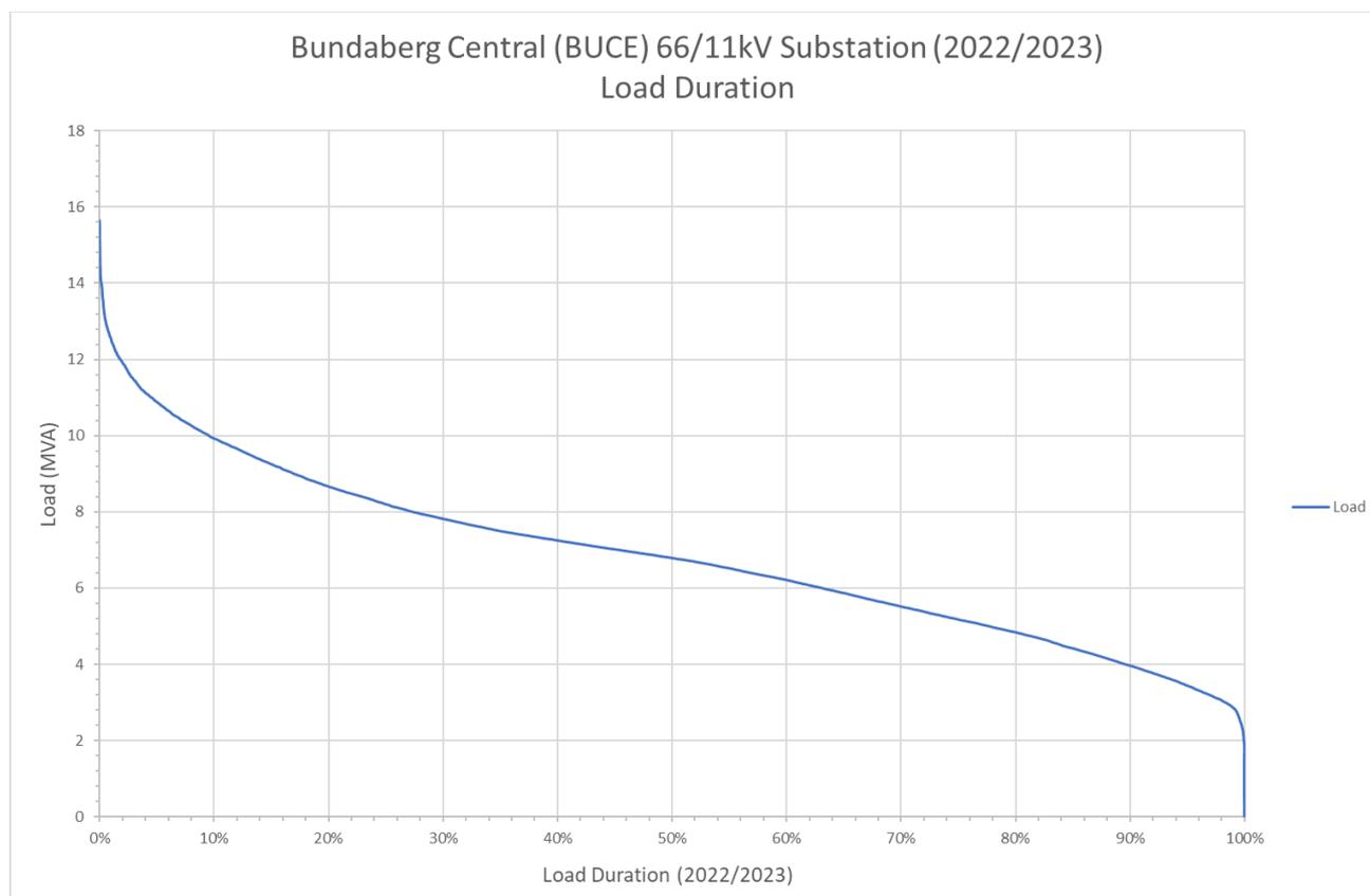
**Figure 9: Bundaberg Central Substation load duration curve**
