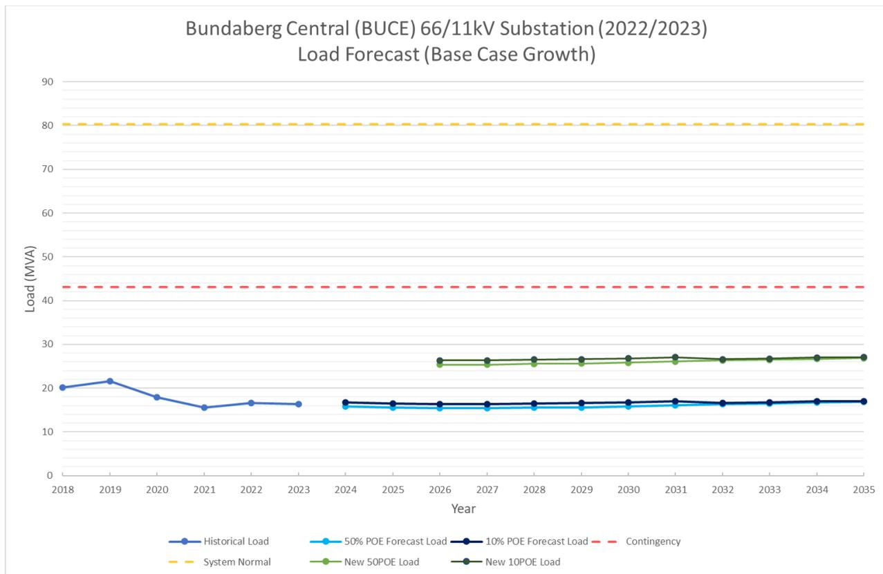
**Figure 17: Bundaberg Central Substation base case load forecast**
