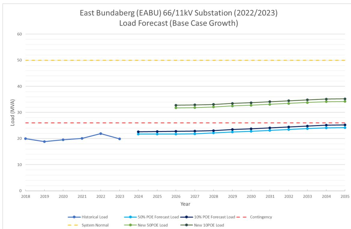
**Figure 18: East Bundaberg Substation base case load forecast**
