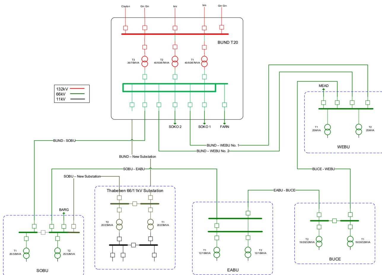
Figure 28: Option A proposed network arrangement (schematic view)
