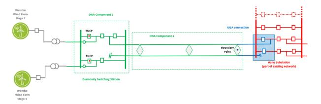
**Note**: The blue shaded area represents the IUSA Component at Halys Substation used to provide negotiated transmission services and does not form part of the Western Downs DNA, but is inherently required in order to connect the Western Downs DNA to the transmission network and is noted in Appendix F of this Access Policy in order for Applicants to have full transparency on costs of access and connection.
