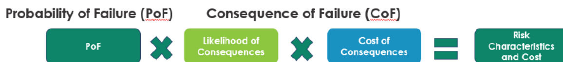
Figure A.2 AusNet’s quantifying asset failure risk approach
