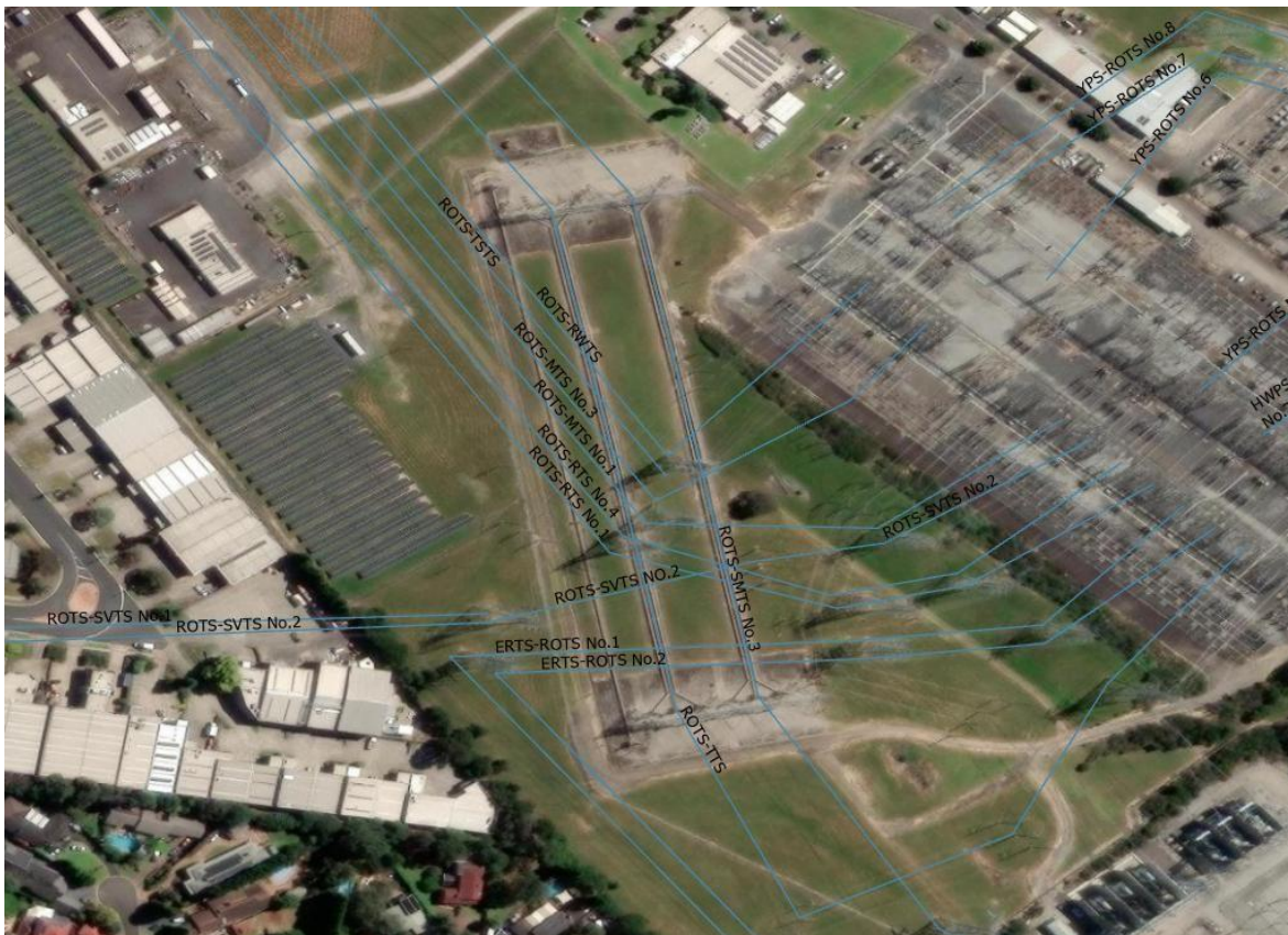
Figure 1: Gas Insulated Lines (GIL) at Rowville Terminal Station
