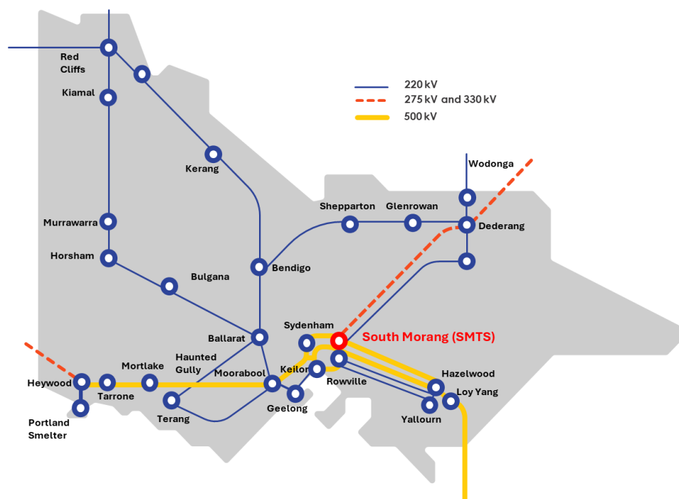
Figure 1: SMTS and the Victorian Transmission network
