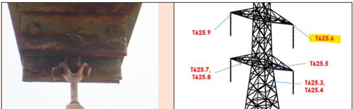
Figure 24: T625 suspension plates, middle phase
