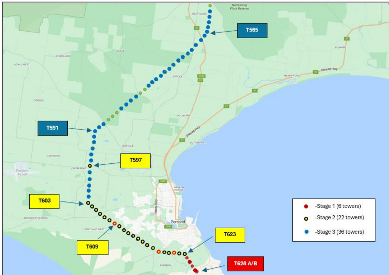
Figure 34: HYTS-APD 500kV line Program Stages 1, 2, and 3
