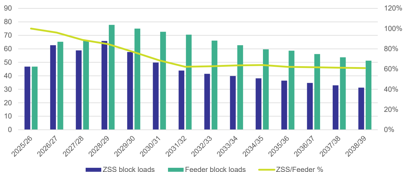
Figure 3-12: Block loads (MW) at the zone substation and feeder level – AusNet growth corridors
