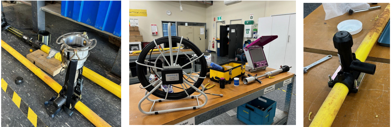
Figure 2.4: Image of new DN40 camera equipment and tees
