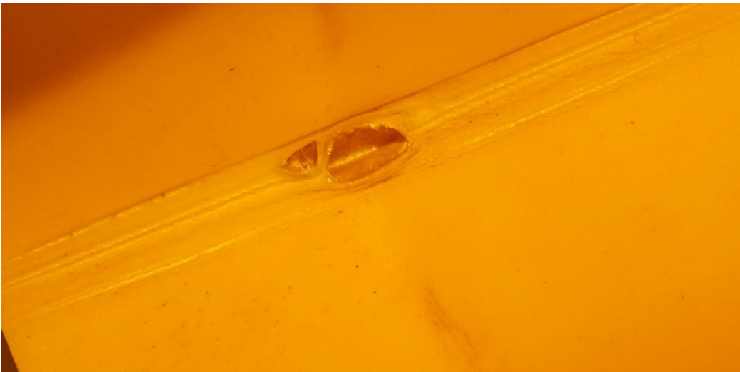
Figure 2.1: Image of a partial crack at an old squeeze off location
