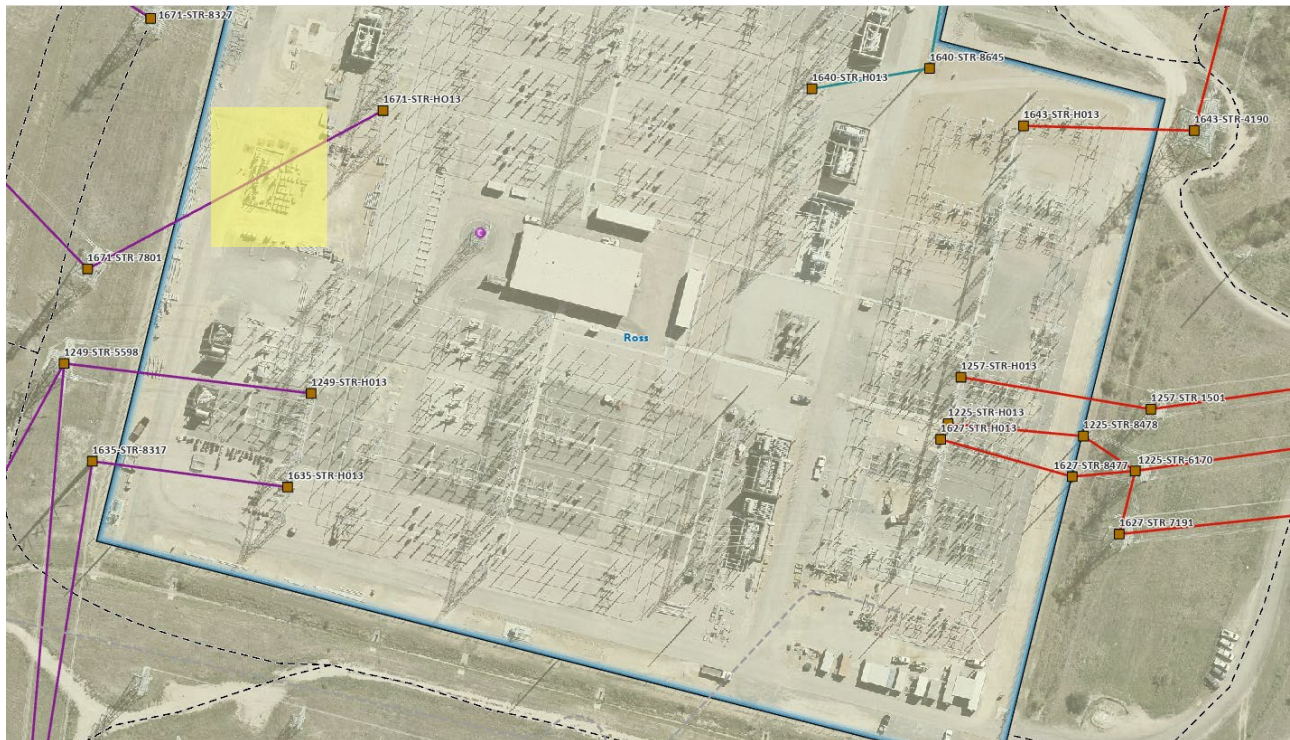
Figure 2 - Proposed location for second spare transformer at H013 Ross Substation
