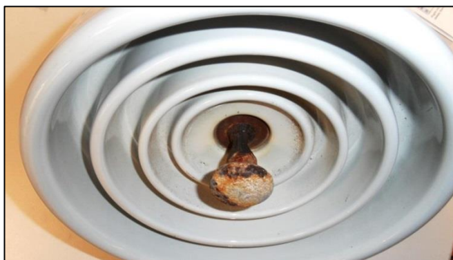
Figure 3: Condition of Removed suspension Insulators
