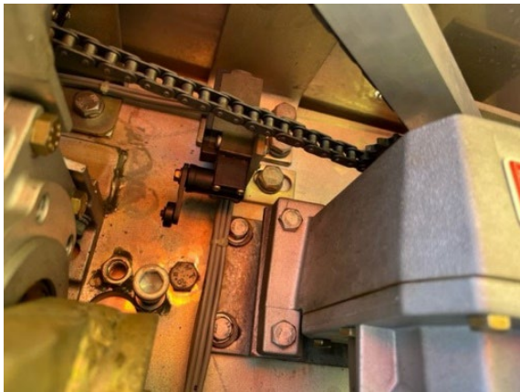
Figure 6--Limit switch and chain drive assembly
