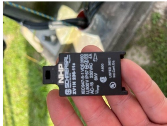
Figure 7-Removed NHP limit switch component
