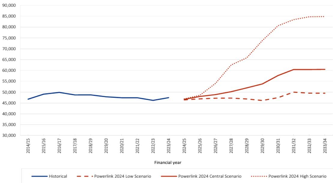
The following graph illustrates the corresponding range of maximum demand, in MW, due to the forecast of energy supplied. The forecast increase in maximum demand ranges between approximately 15% and 70% over the 10 years to 2033/34.
