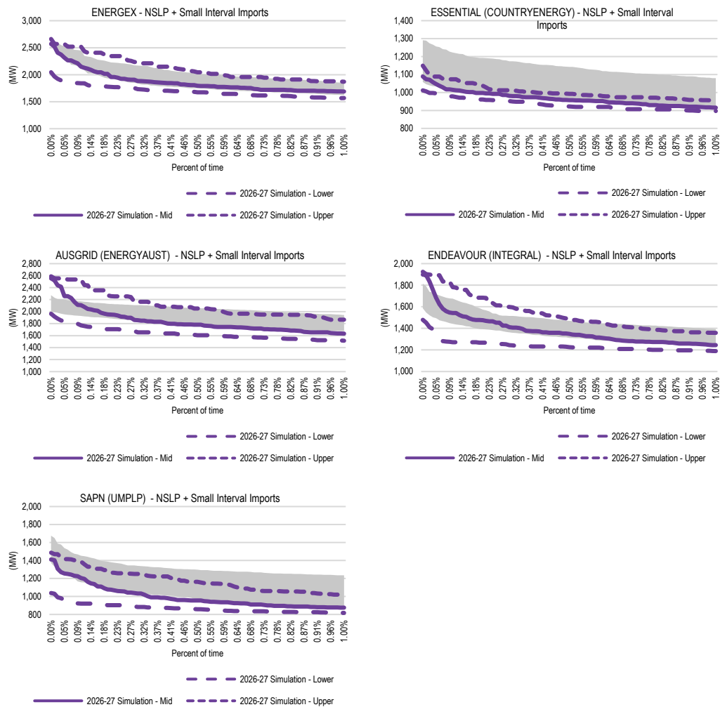
Figure 3.14 Comparison of upper one per cent of hourly NSLP and small interval meter import demands of 2026-27 simulated hourly demand sets with historical outcomes
