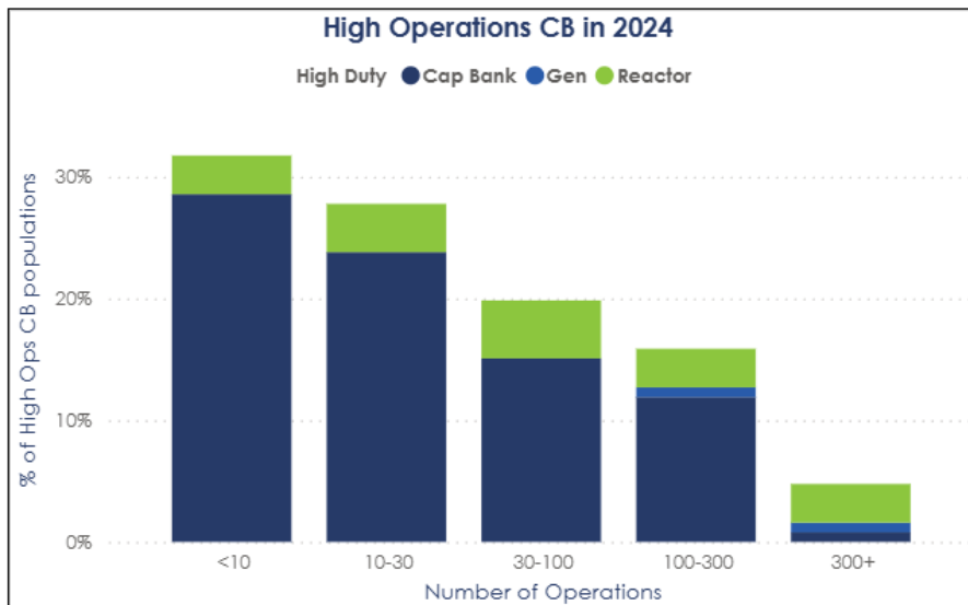
Figure 13: Capacitor bank, Generation & Shunt Reactor CB operation graph in 2024
