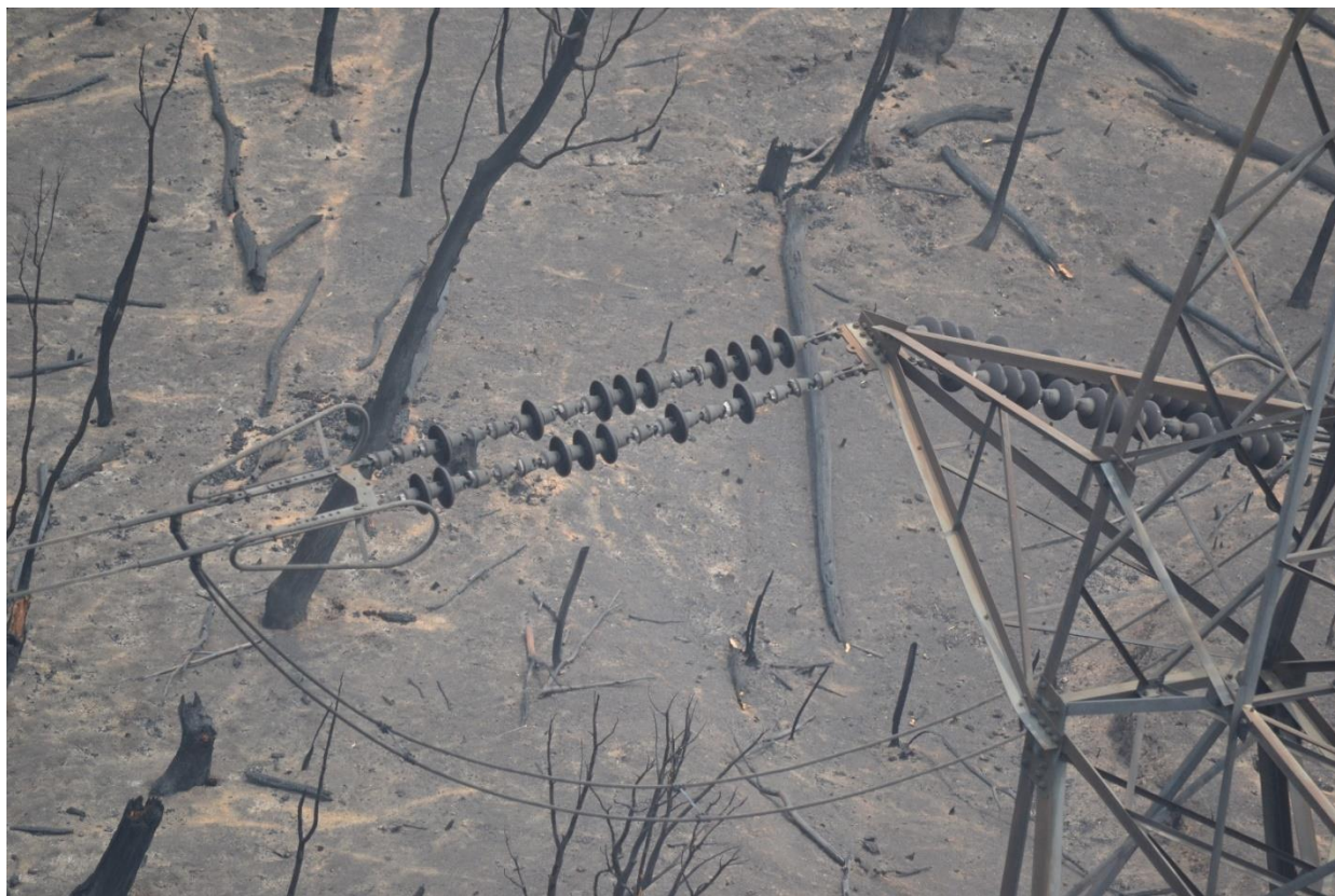
Figure 11 – Line 2 Damaged Insulators
