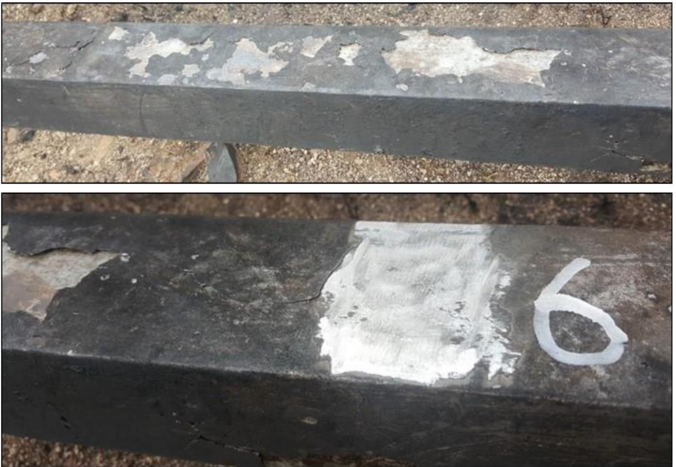
Figure 27 – Flaking of galvanising on the surface of a structure on Line U3
