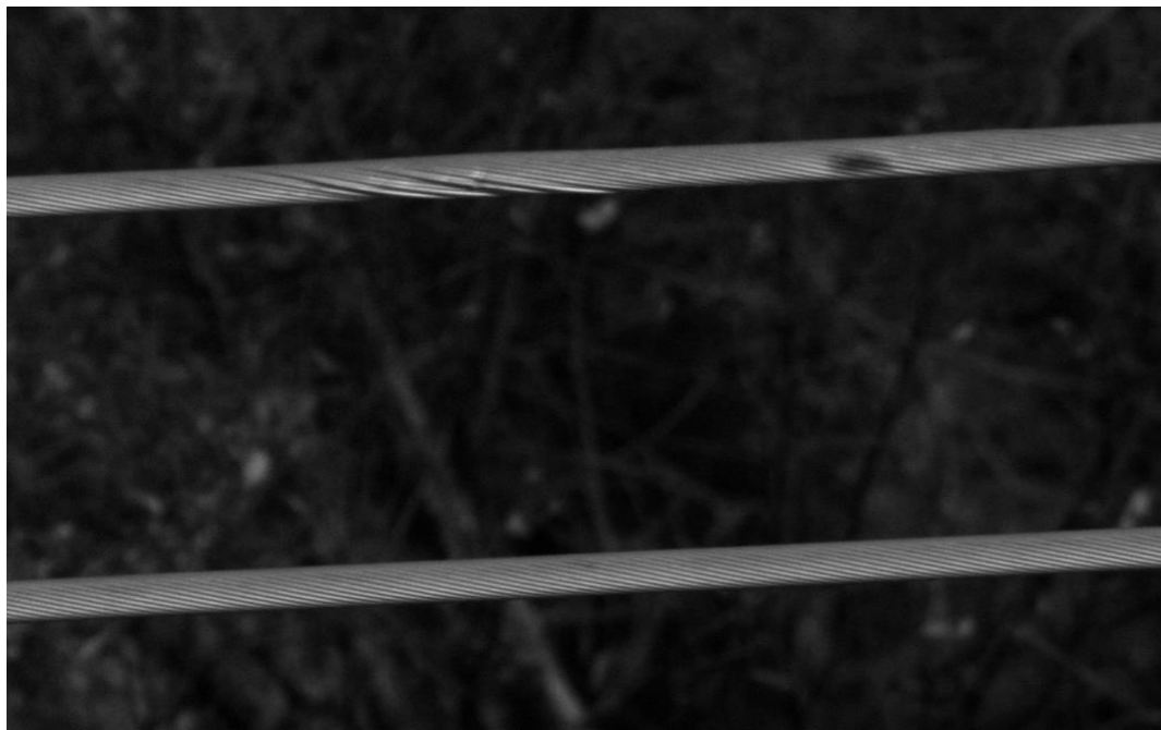
Figure 39 – ACSR conductor damage – loose strands
