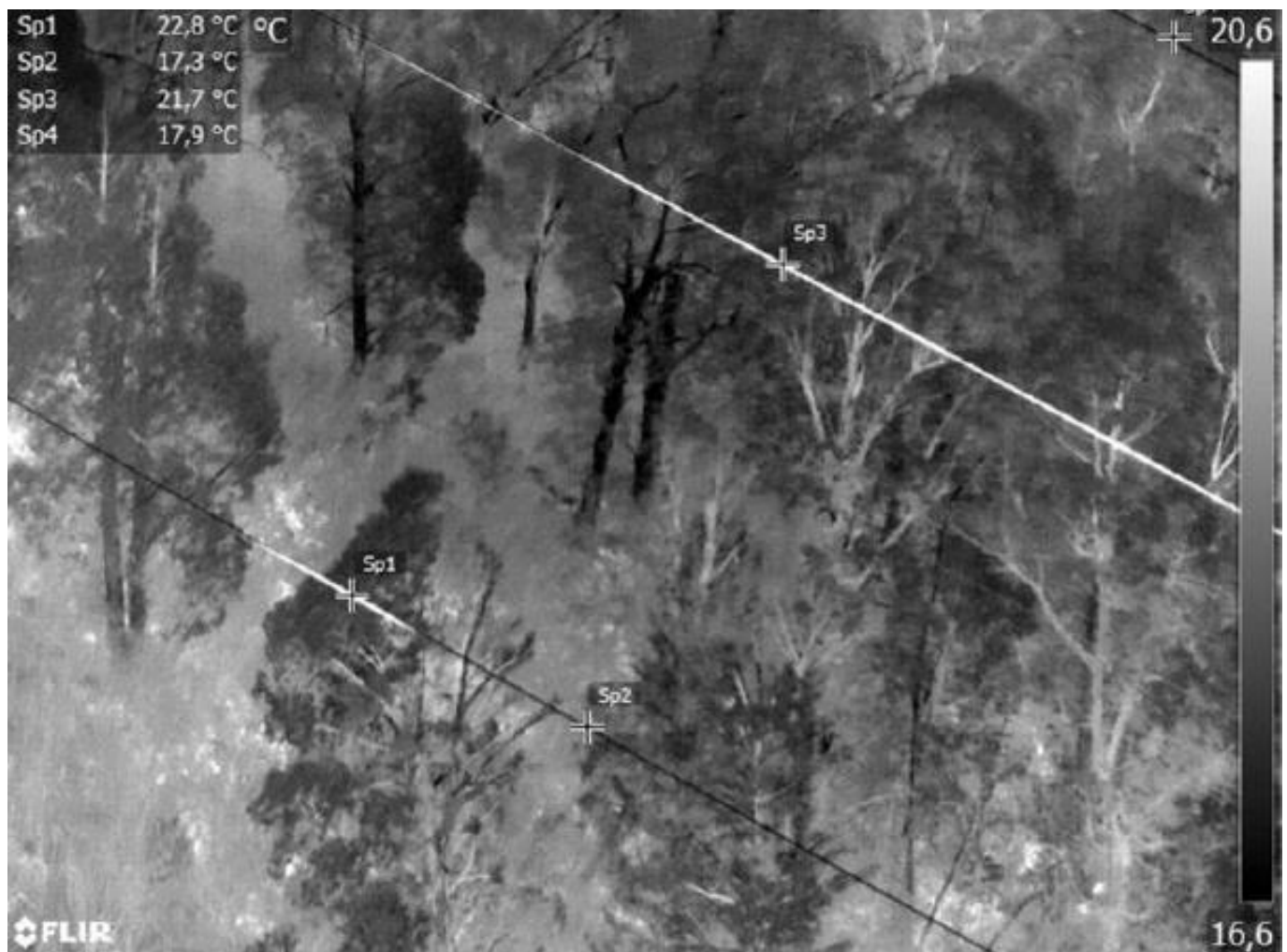
Figure 38 - Conductor damage example of 'hot spots' [REDACTED] identified in multispectral (IR) inspection
