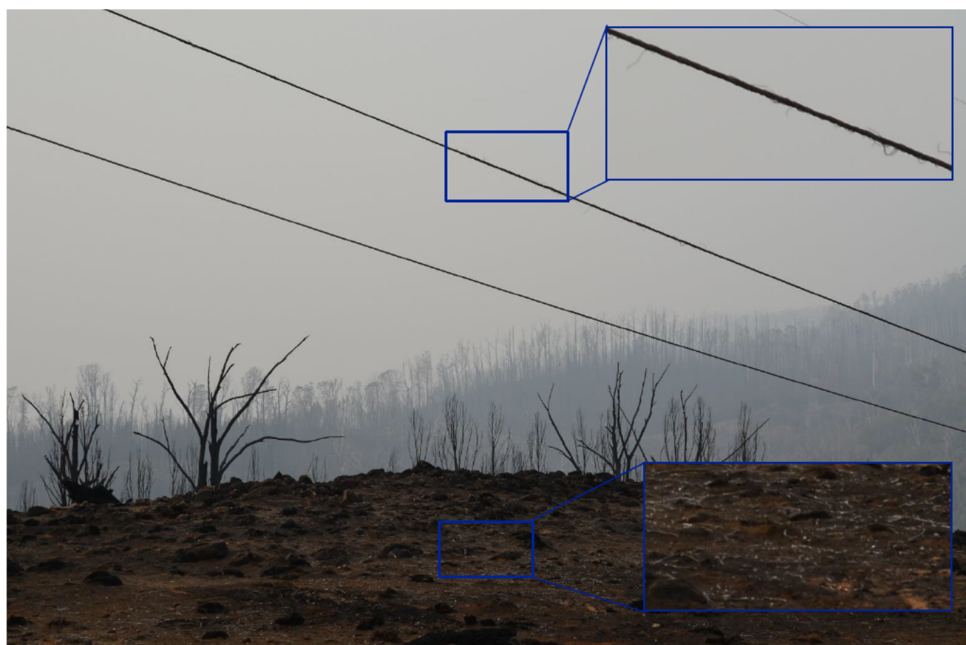
Figure 33 - Extensive conductor damage with melted aluminium
