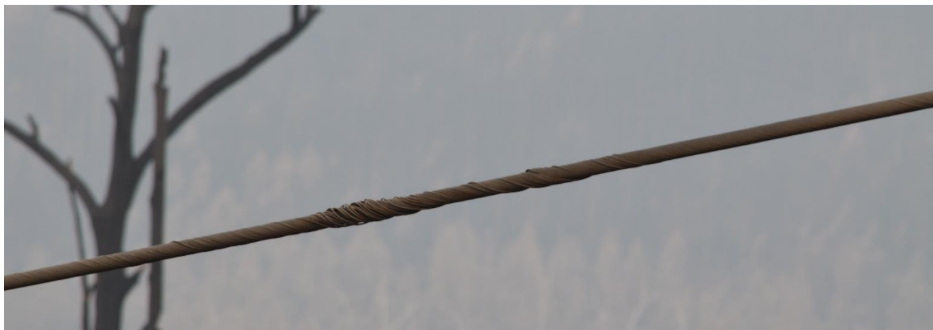
Figure 37 – Conductor damage example on AAAC conductor [REDACTED] identified visually
