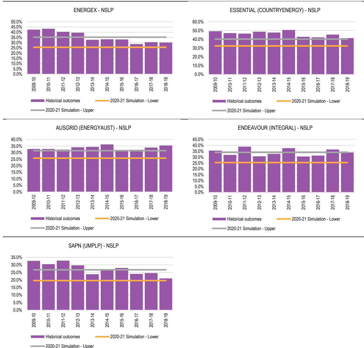
FIGURE 4.18 COMPARISON OF LOAD FACTOR OF 2020-21 SIMULATED HOURLY DEMAND DURATION CURVES AND HISTORICAL OUTCOMES - NSLPS
