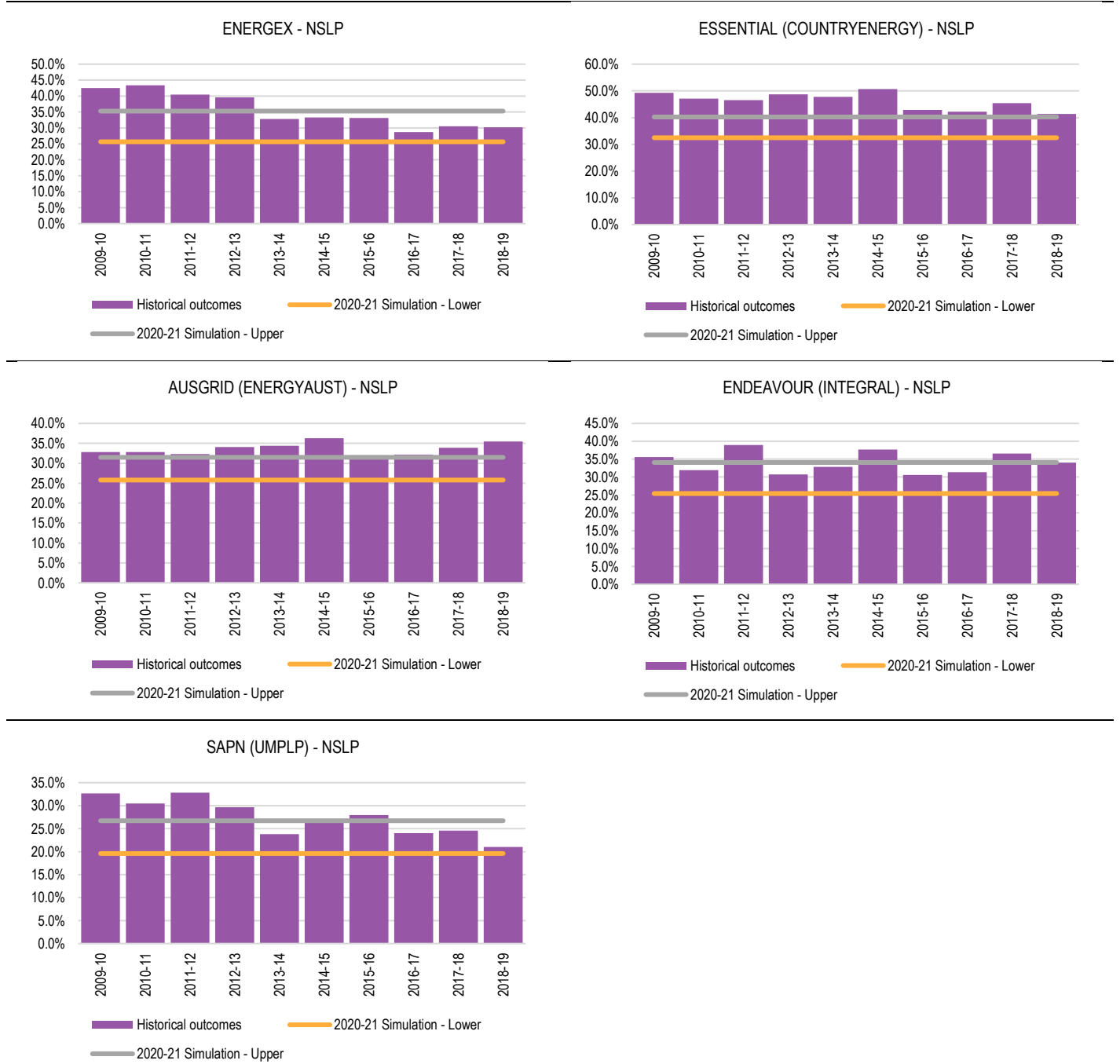
FIGURE 4.18 COMPARISON OF LOAD FACTOR OF 2020-21 SIMULATED HOURLY DEMAND DURATION CURVES AND HISTORICAL OUTCOMES - NSLPS
