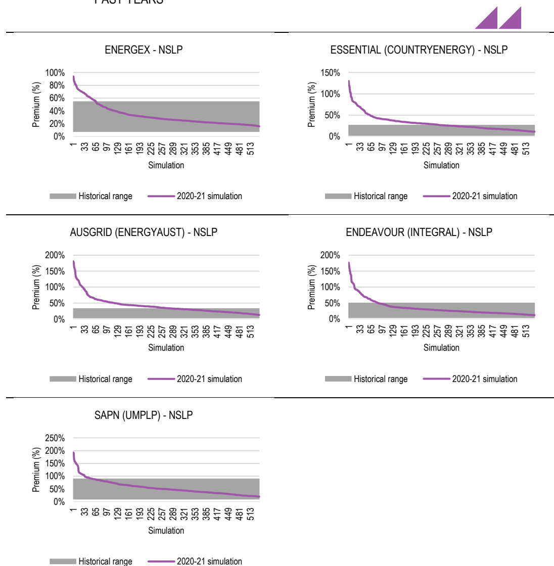
FIGURE 4.22 ANNUAL DWP FOR NSLP AS PERCENTAGE PREMIUM OF ANNUAL TWP FOR 539 SIMULATIONS FOR 2020-21 COMPARED WITH RANGE OF ACTUAL OUTCOMES IN PAST YEARS
