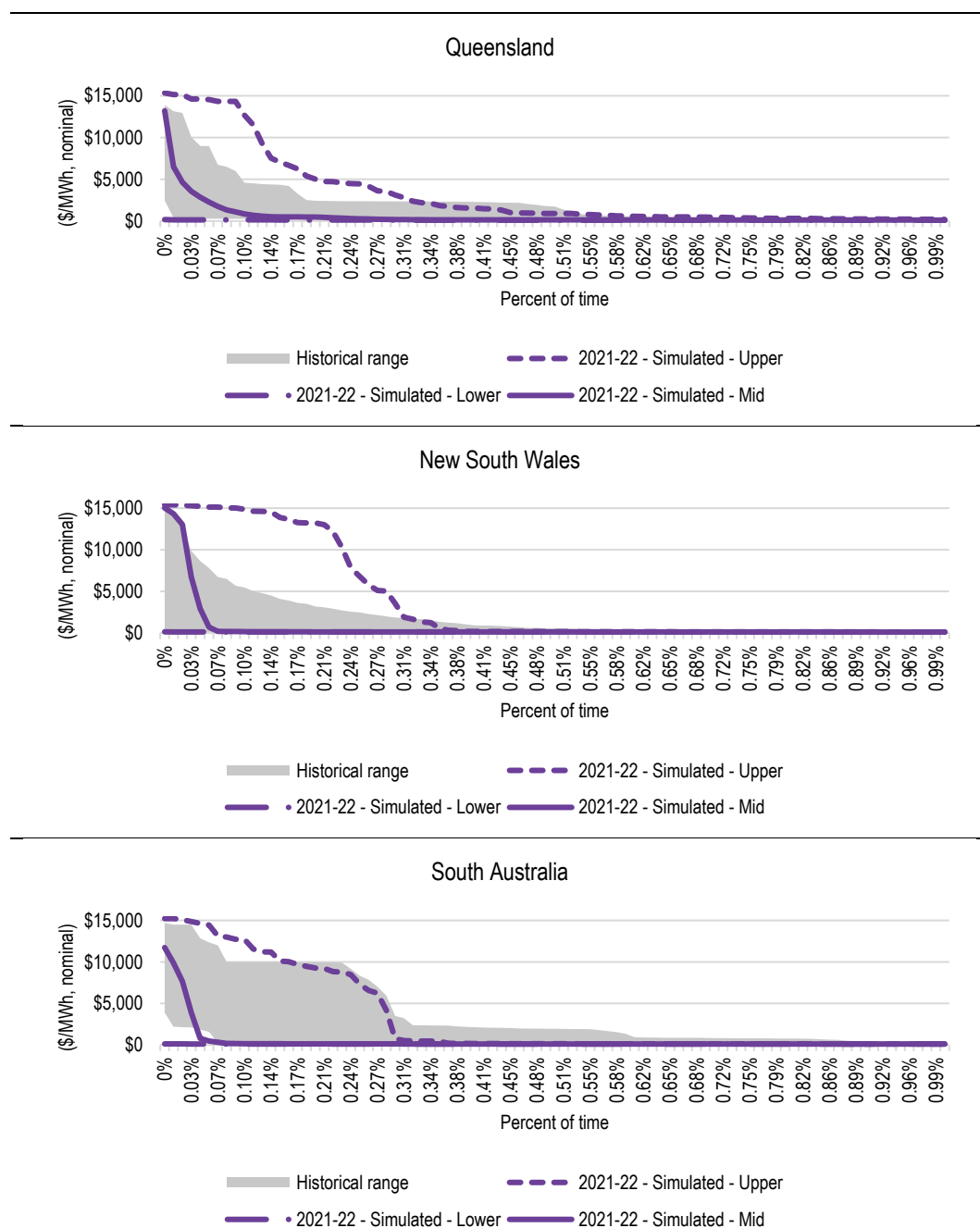
Figure 4.21 Comparison of upper 1 percent tail of simulated hourly price duration curves for Queensland, New South Wales, and South Australia for 2021-22 and range of actual outcomes in past years
