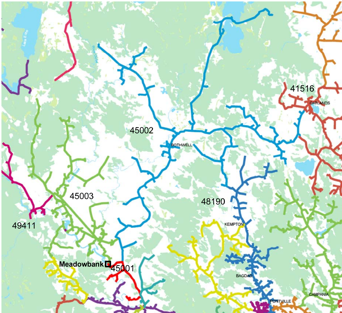
Figure 8-11 Meadowbank 22 kV feeders
