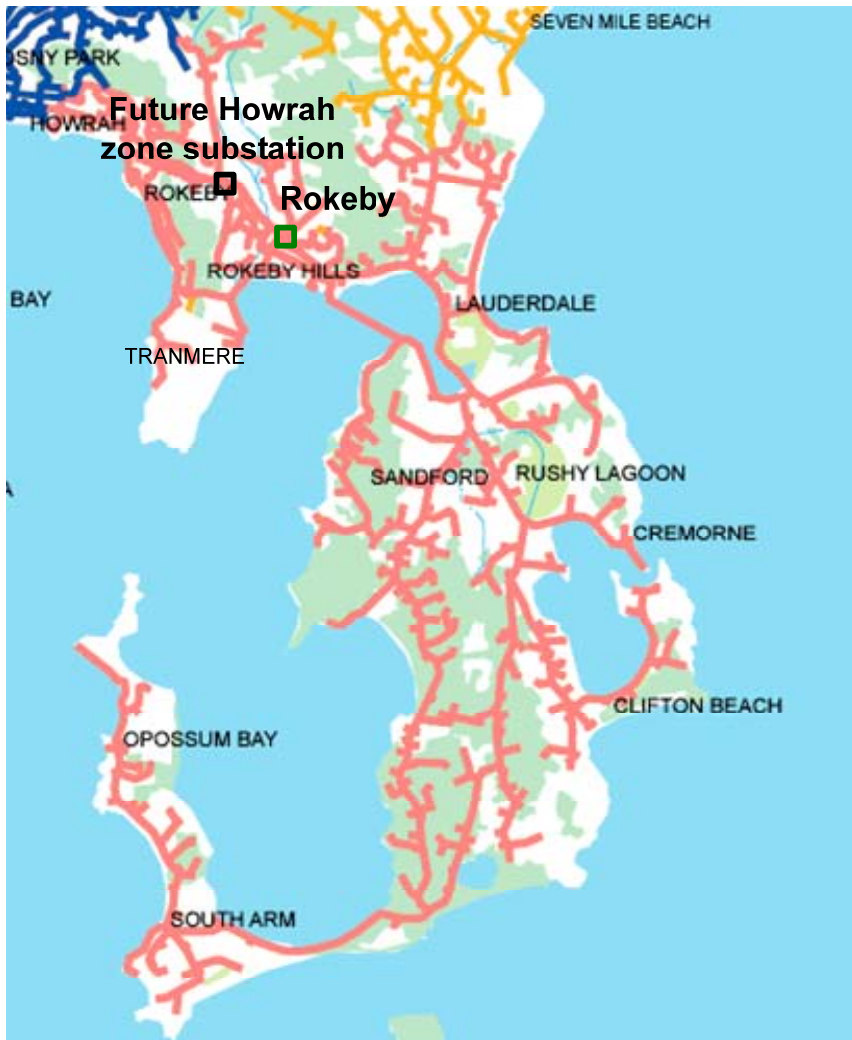
Figure 8-22 Rokeby 11 kV supply area
