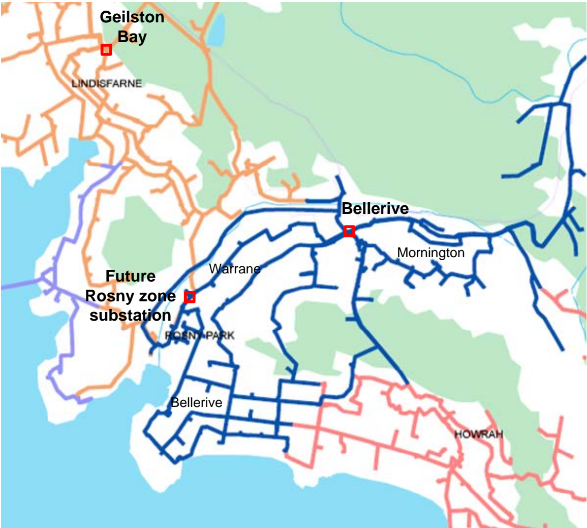
Figure 8-11 Bellerive 11 kV supply area
