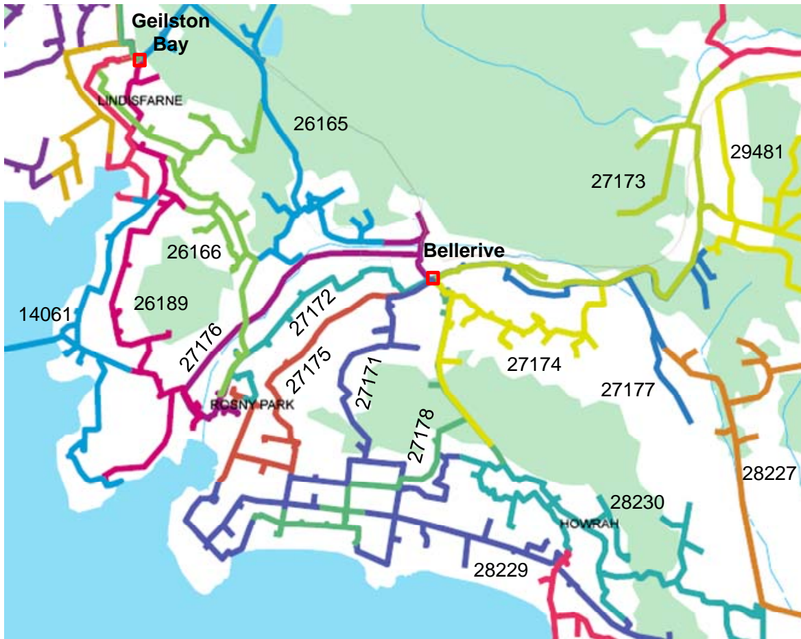
Figure 8-12 Bellerive 11 kV feeders
