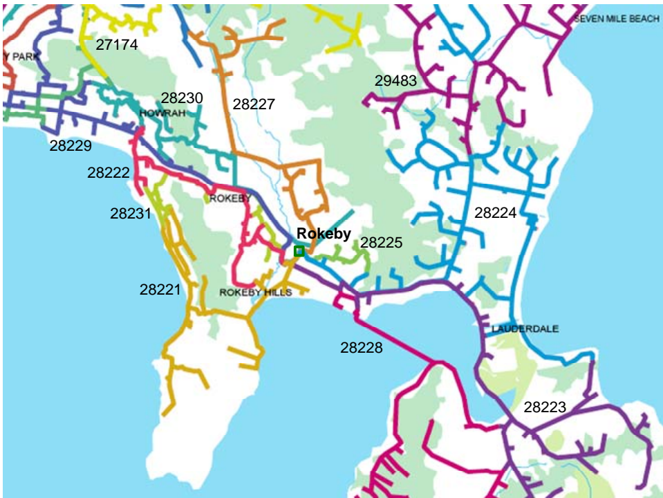
Figure 8-23 Rokeby northern 11 kV feeders
