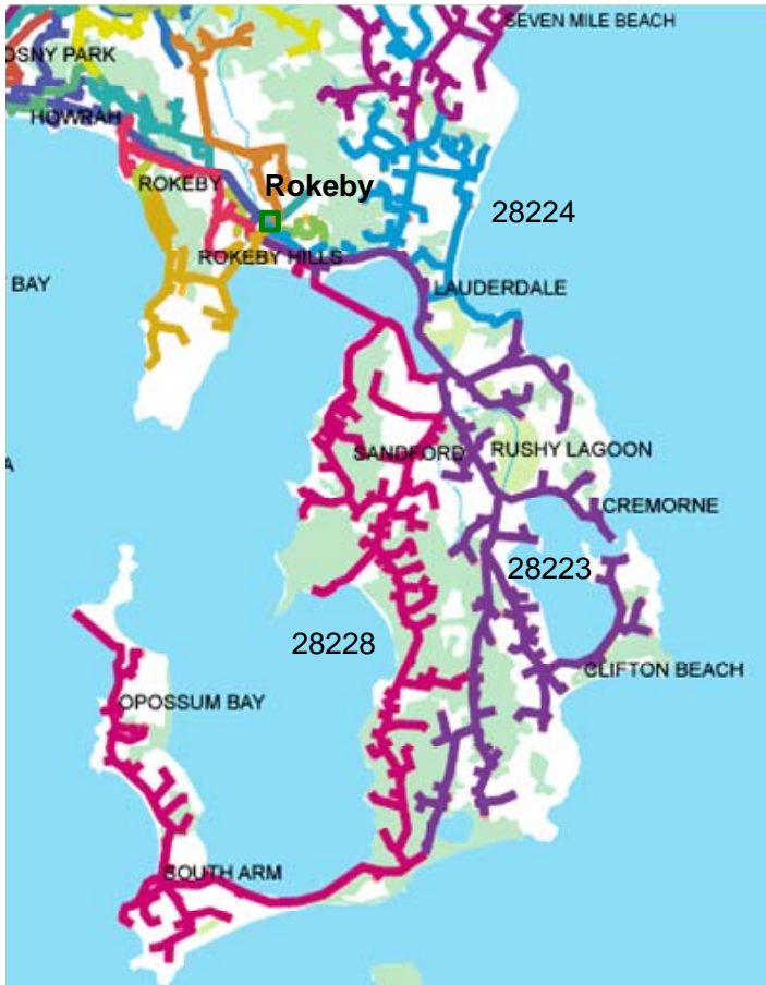
Figure 8-24 Rokeby southern 11 kV feeders
