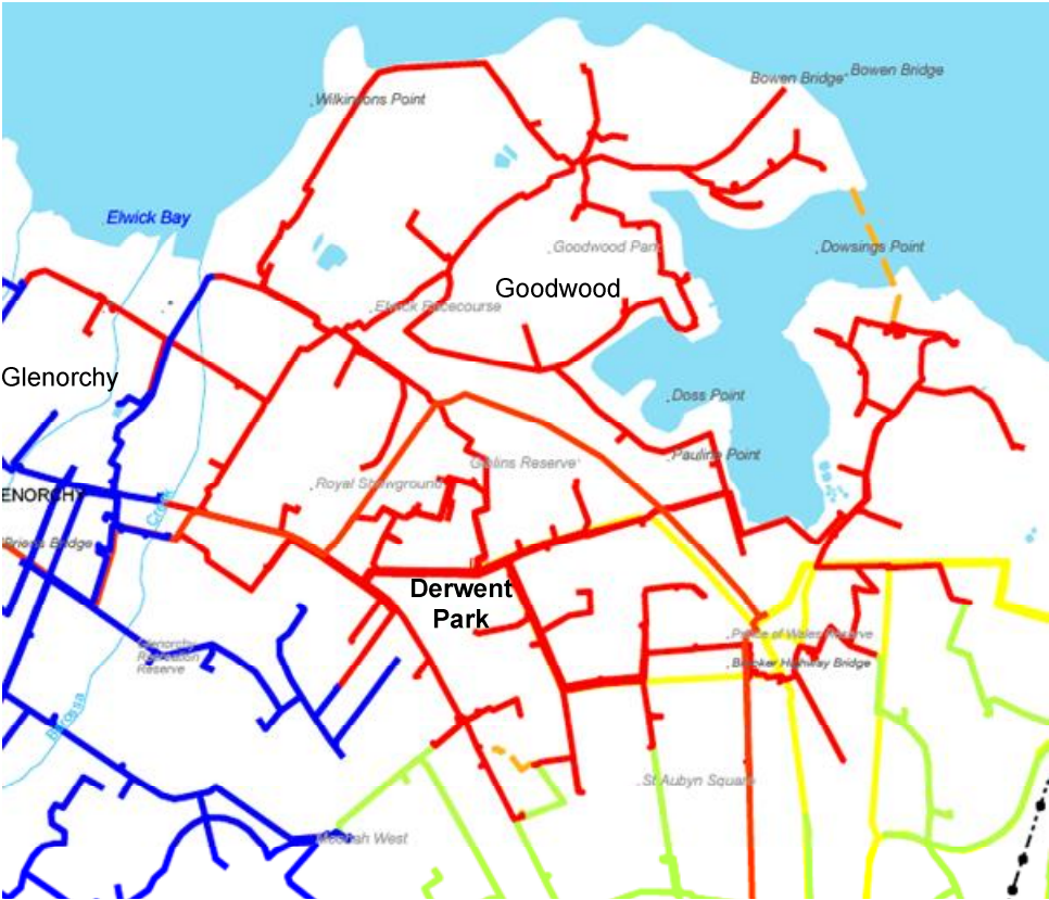
Figure 8-14 Derwent Park 11 kV supply area
