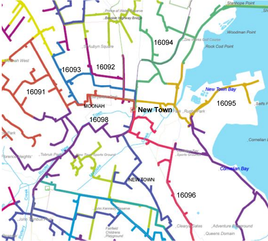
Figure 8-18 New Town 11 kV feeders
