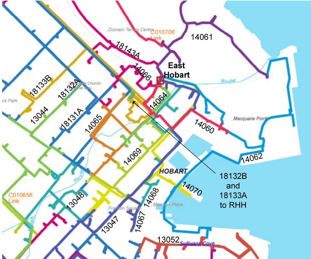
Figure 8-29 East Hobart 11 kV feeders
