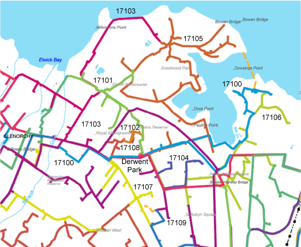
Figure 8-15 Derwent Park 11 kV feeders
