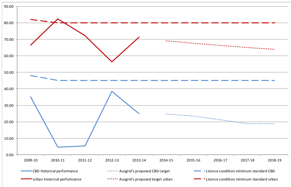
Figure 11-1 Ausgrid's unplanned SAIDI performance, proposed target and minimum standards for CBD and urban areas (minutes)
