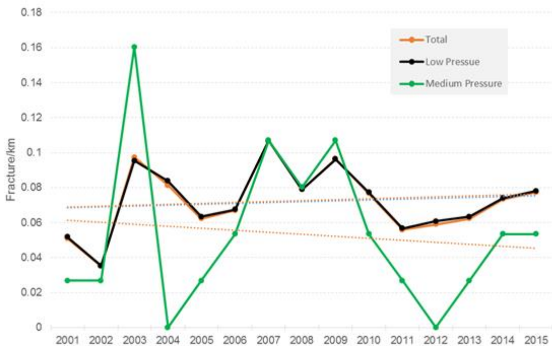
Figure 6.3 Distribution mains cast iron fracture incident rate
