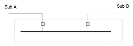
Step 3.2: The stand-alone arrangement for the provision of *prescribed common transmission services* to an equivalent standard is shown below and consists of 3 circuit breakers.
