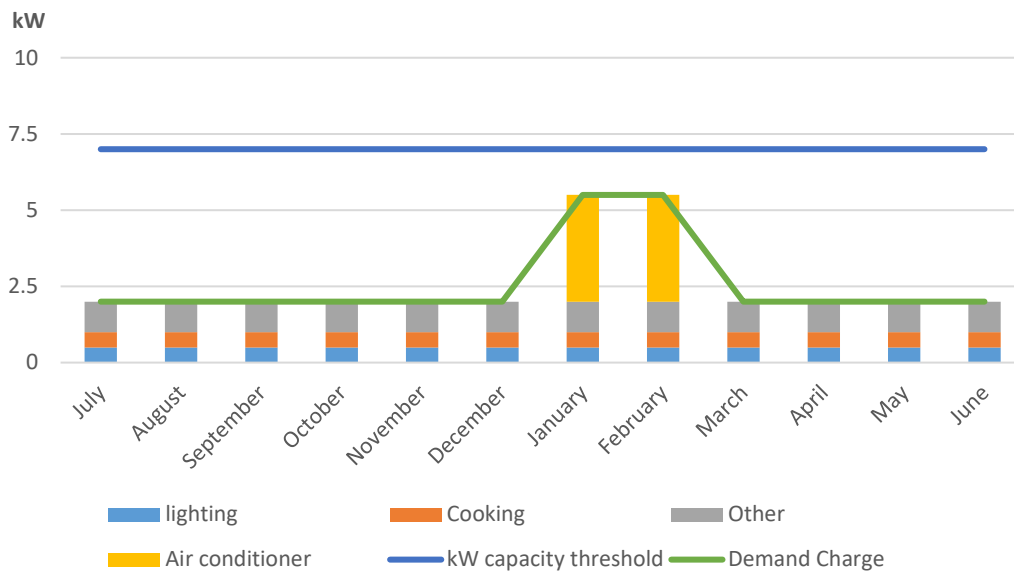
Figure 18.2 Illustrative example - capacity charge Vs demand charge
