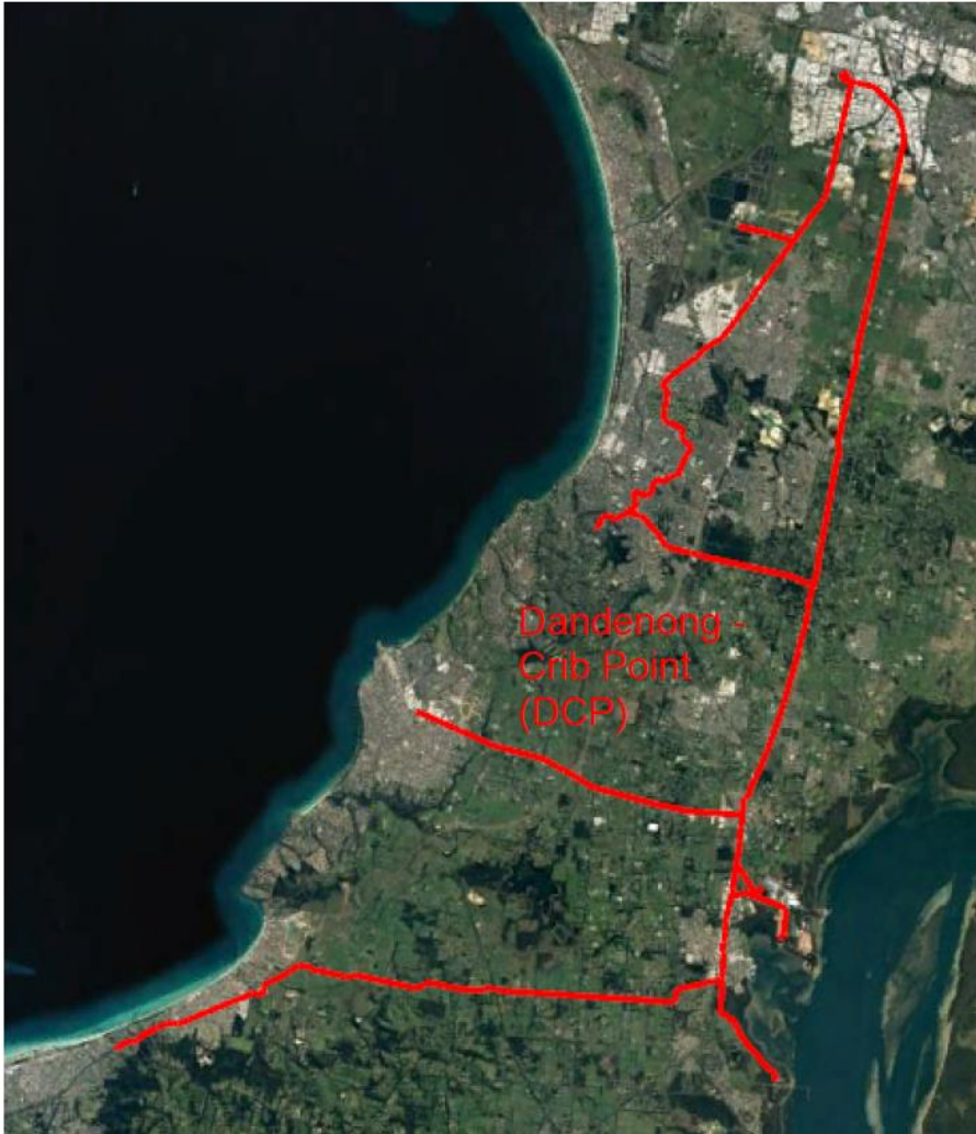
Figure 1-3: VIC TP pipeline network
