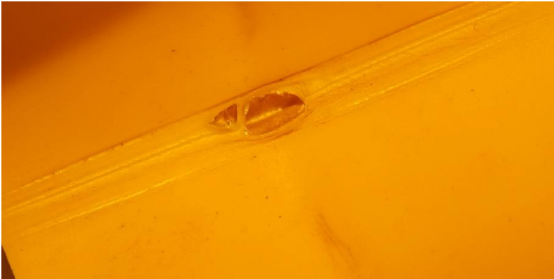
Figure 4: Image of a partial crack at an old squeeze-off location
