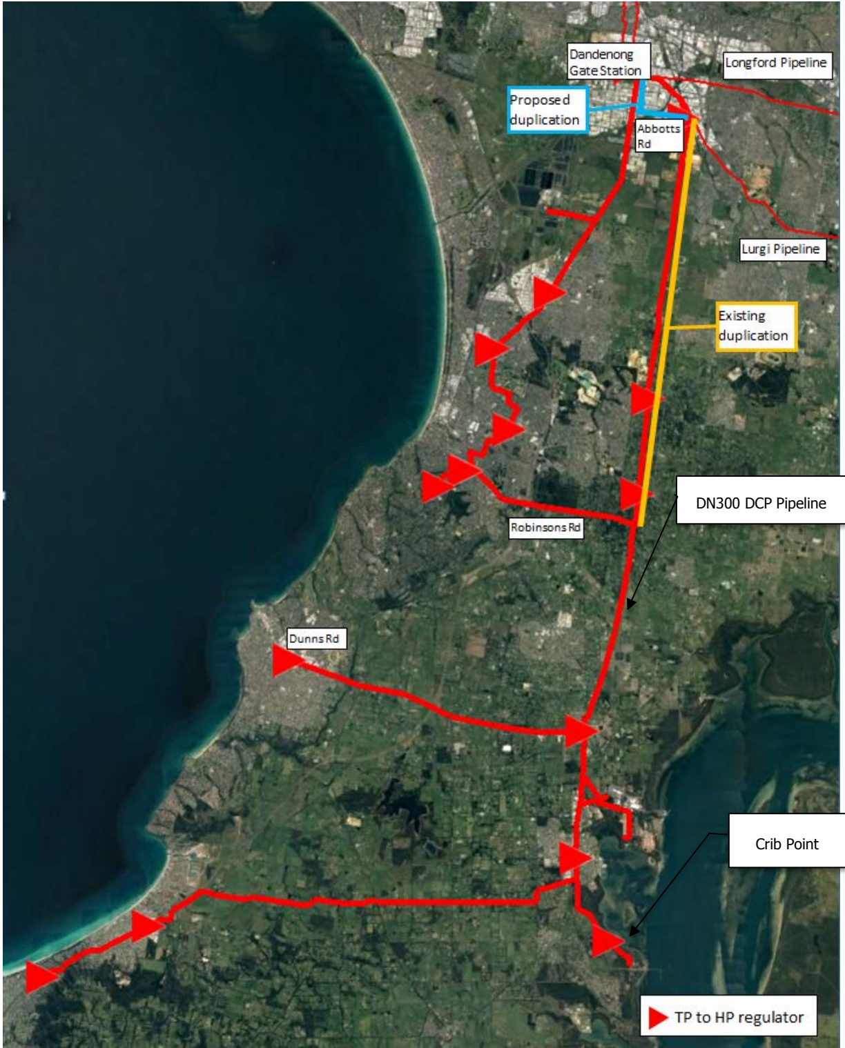
Figure A.1 – Dandenong Crib Point Transmission Pipeline
