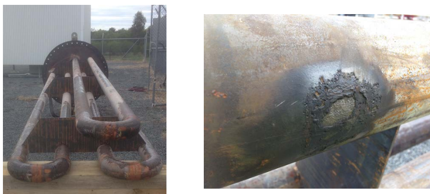
Figure 1.1: Typical Corrosion of Coils Resulting in End-of-Life Assessment
