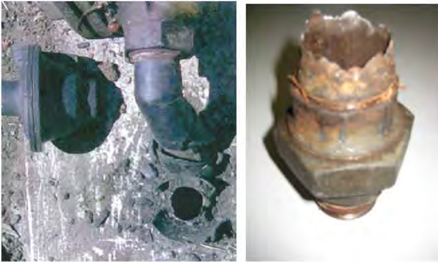
Figure 1.3: I&C meter set corrosion – soil/air interface
