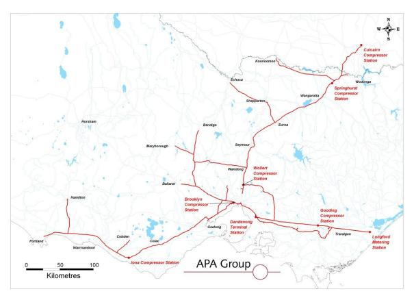
Gas enters and exits the system in the West via the SeaGas connection point and Western Underground Storage (WUGS) facility at Iona, to the North via the APA GasNet Northern Lateral Pipeline at Culcairn and to the East from Longford, VicHub and Bass Gas.
