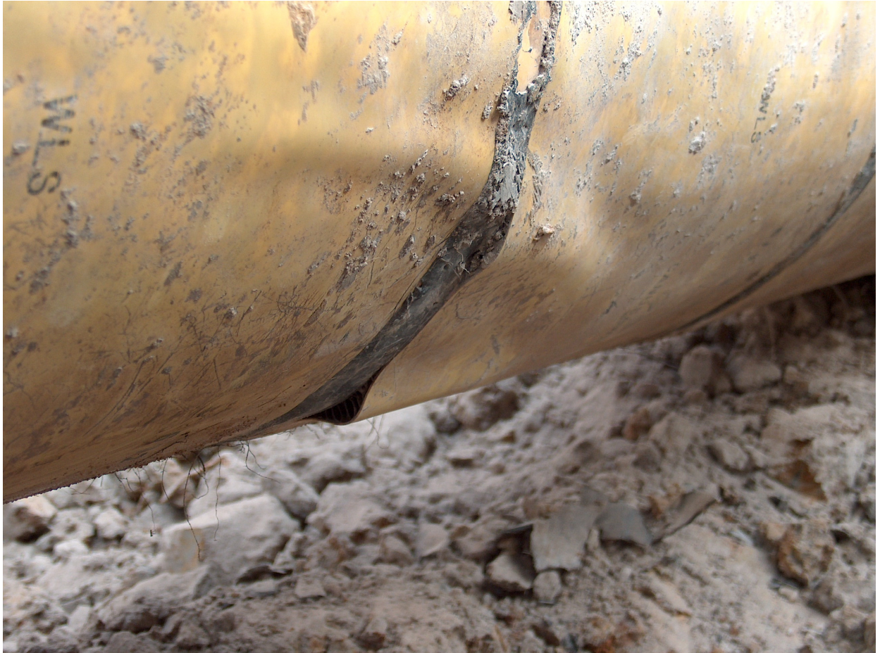
Image 2: The disbonded heat shrink sleeve is clearly evident on visual inspection
