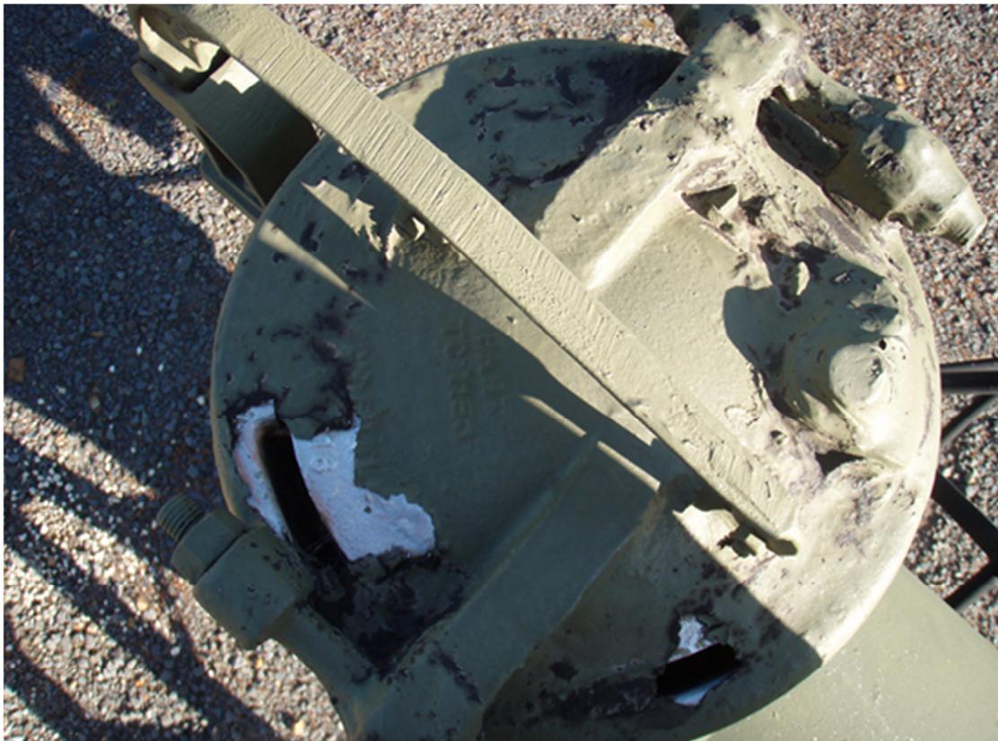
Picture shows the Unibolt enclosures ability to hold water and corrode.
