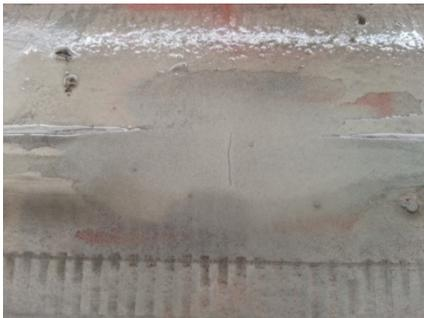
Further investigation was carried out with ultrasonic non-destructive testing to determine the extent of the crack. Results confirmed the crack was 4.5mm deep and approximately 12mm long across the longitudinal seam weld.
