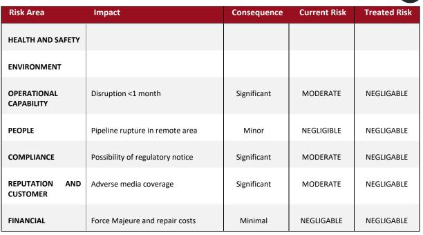
The risk assessment indicates that there is a moderate risk, resulting from the failure to replace obsolete CP units pro-actively to ensure that CP is controlled to the desired level to resist corrosion.
