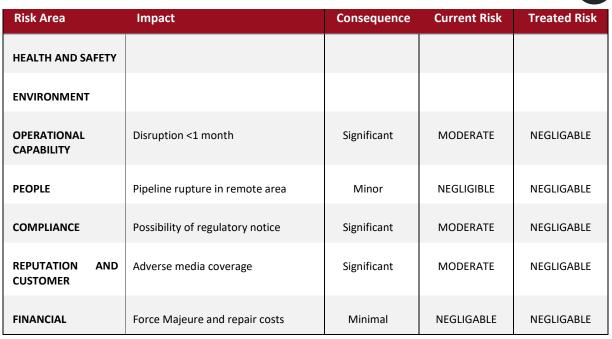
The risk assessment indicates that there is a moderate risk, as the likelihood of total power failure from a solar site is low and whilst the site may fail daily the time for extensive corrosion to occur would be significant. This would not be in compliance with AS2885.1 section 6.4.4 that requires "...satisfactory protection ... with timely and appropriate action to restore full protection..."
