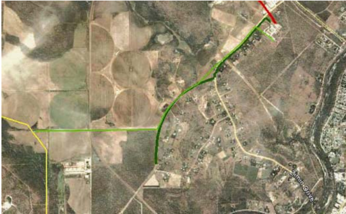
Figure 4.1 Katherine lateral pipeline (light green) and powerline alignment (dark green), with AGP in lower left (bright yellow).
