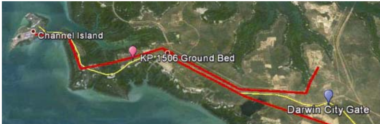
Figure 4.3 Channel Island spurline (yellow) and 132 kV powerlines (red).
