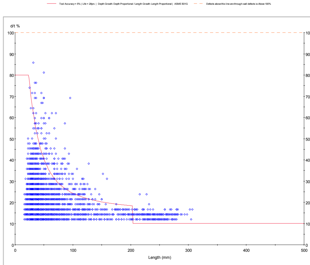
Figure B.22 Renner Springs – Newcastle Waters – 5.8 mm WT - Anomaly Proportional Growth - ASME B31G - Year 2036
