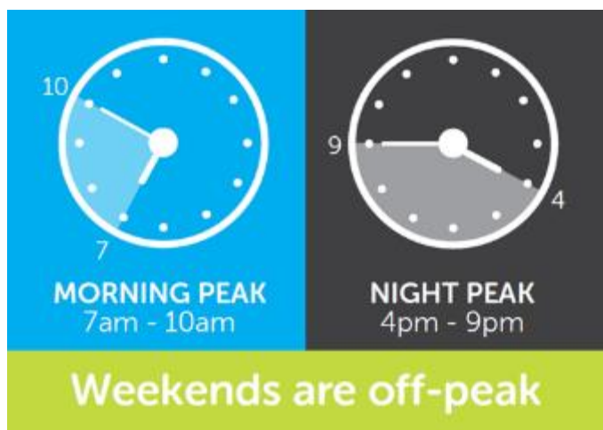
Figure 5 – Time of use periods for residential time of use consumption based network tariff (TAS93)
