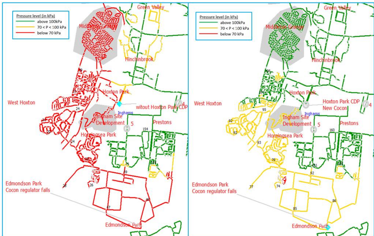
Figure 2–8: Wetherill Park 210 kPa network severe winter peak 2020 under failure of Edmondson Park Regulator – without and with Hoxton Park CDP
