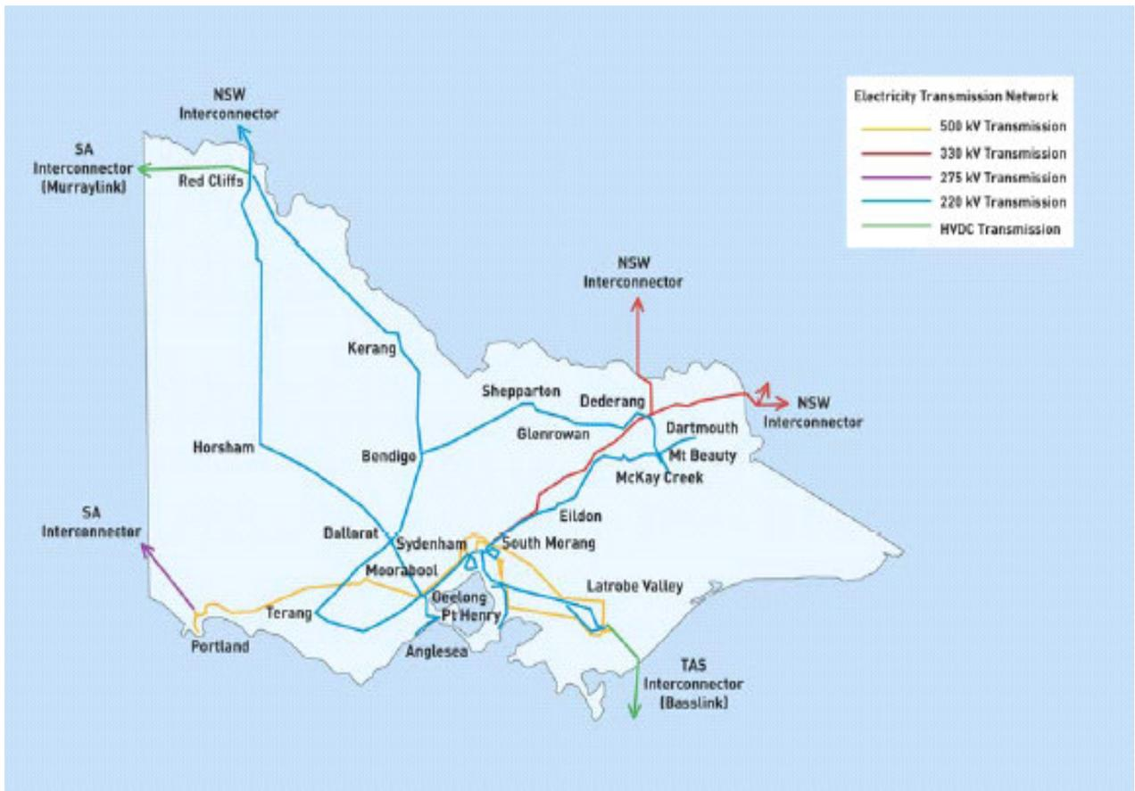
Figure 4 – Victorian Electricity Transmission Network
