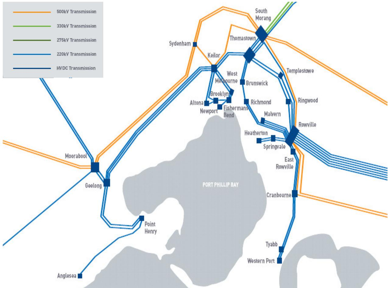
Figure 5 – Metropolitan Melbourne Electricity Transmission Network
