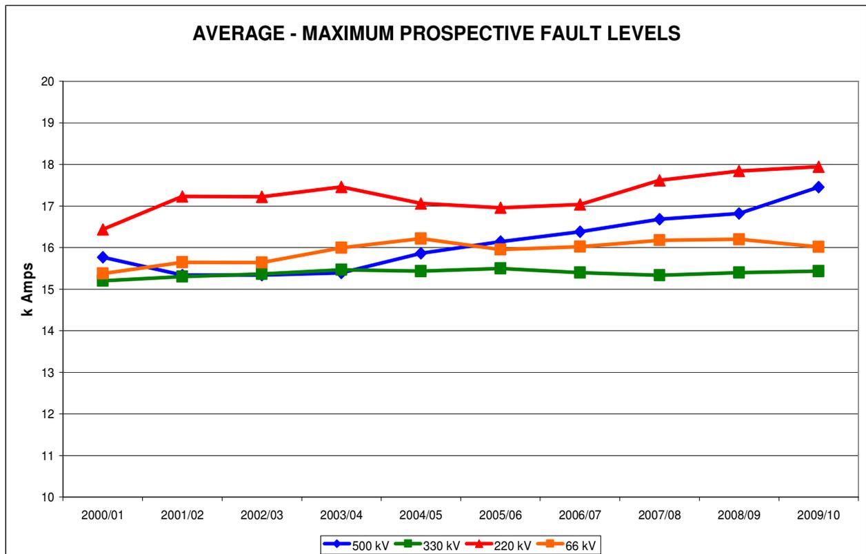
Figure 19 – Average Maximum Prospective Fault Levels
