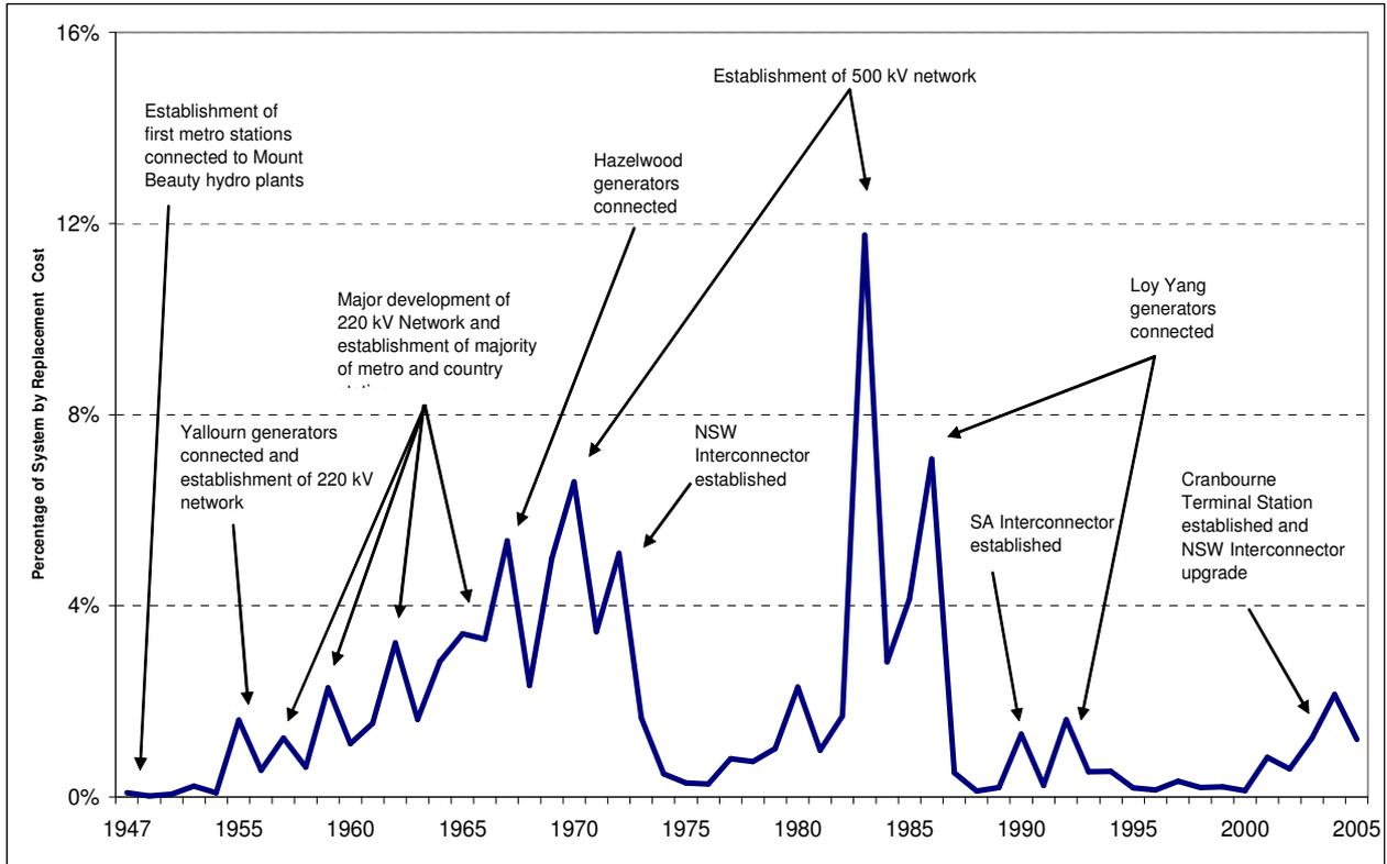
Figure 7 – Development of the Victorian Electricity Transmission Network
