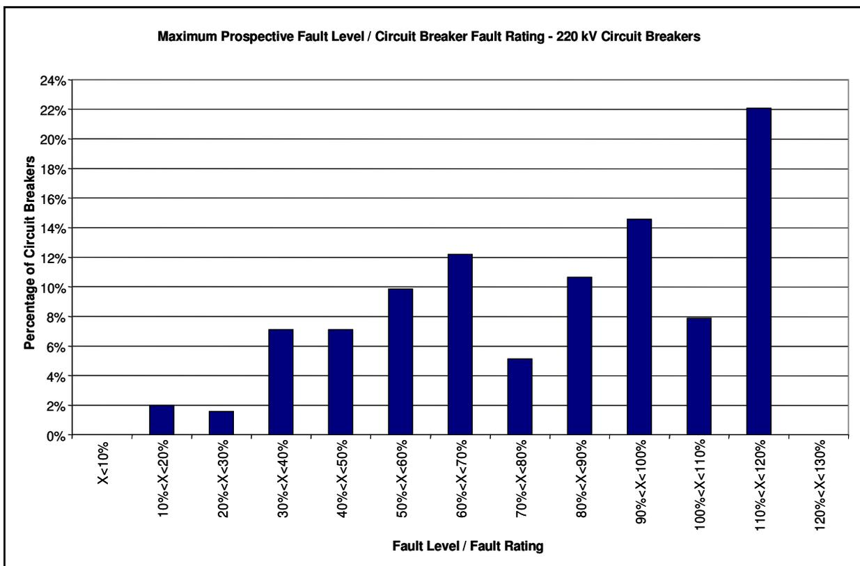
Figure 33 – 220 kV CBs X Fault Levels 2005
