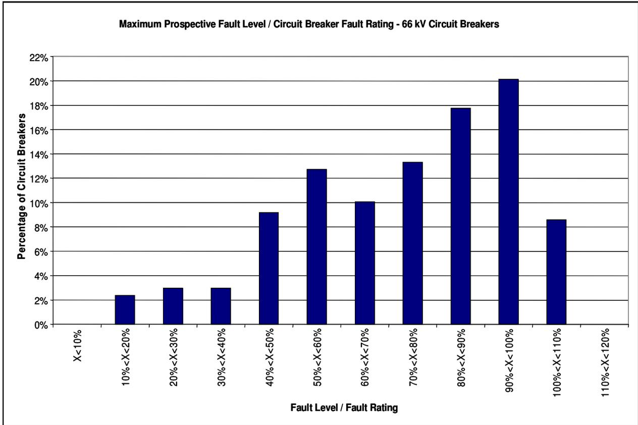
Figure 34 – 66 kV CBs X Fault Levels 2005
