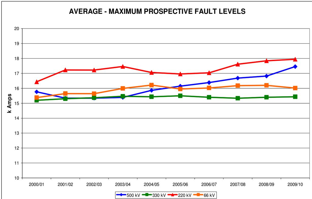
Figure 32 – Average maximum prospective fault levels
