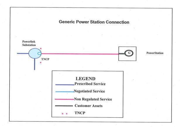
J. The single line diagram above shows each of the prescribed, negotiated and non-regulated services for a generic radial line generator connection to the transmission network. This Negotiating Framework applies only to the provision of Negotiated Transmission Services.
