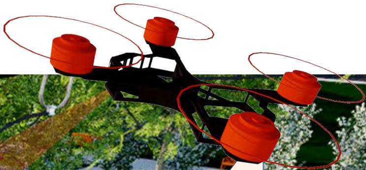
**4** A small inspection drone will be carried by most vehicles, enabling a preliminary check of the network as they arrive at their task location, and aerial views to enable better understanding of the tasks they will be required to perform.
