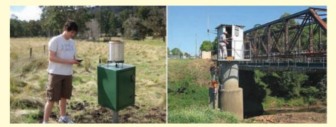
Testing the radio signal from an automatic rain-gauge at Nundle, near the head of the Peel River.
