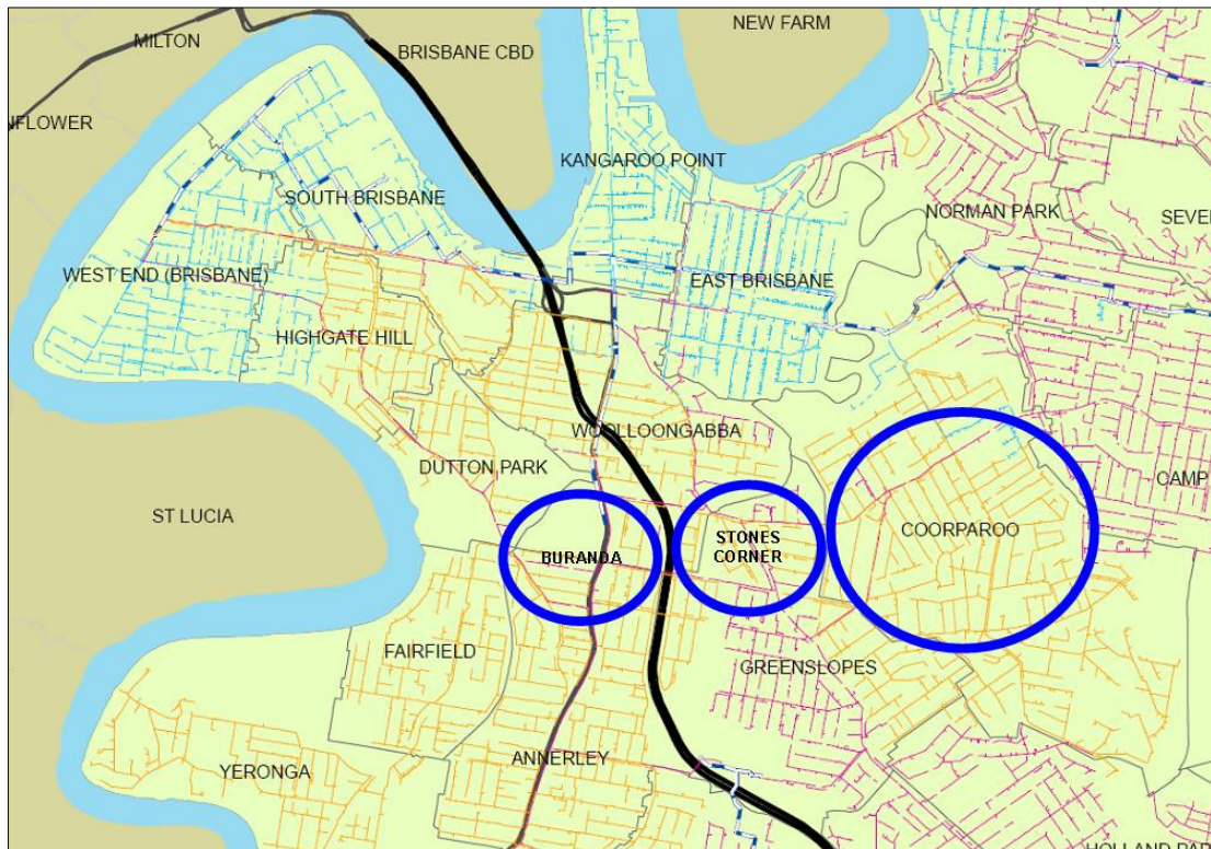
Figure 3-1 APT Allgas network, with identified growth and infill areas
