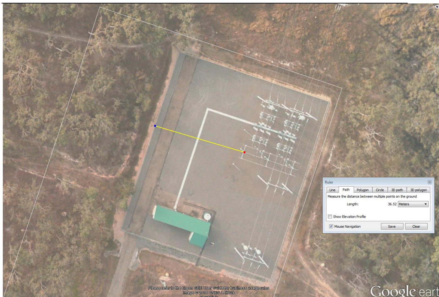
Figure F7: Expand existing yard to North and include additional 3 x 132 kV bays (i.e. 2 x feeder bays, 1 x bus section bay) and a bypass 132 kV bay adjacent 7285 (LAKE).
