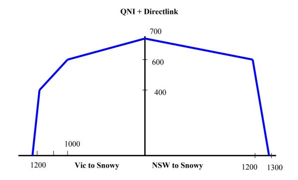
When there is a high power transfer between NSW and Victoria the power transfer capability between NSW and Queensland approaches zero, and vice versa.
