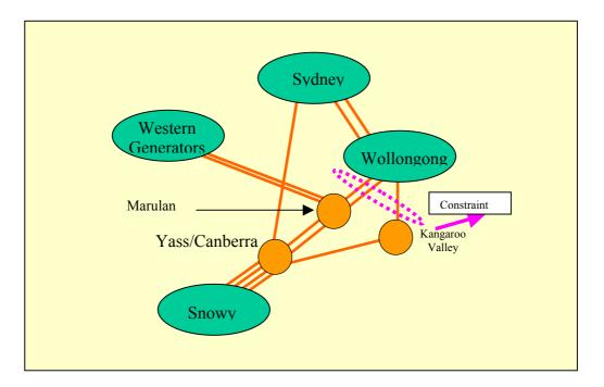
Marulan connects to the south coast system via two 330 kV lines. The south coast is further supported by a 330 kV line from Canberra via Kangaroo Valley and two 330 kV lines from Sydney.
