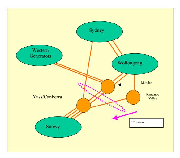
Four 330 kV lines presently extend from Sydney and the south coast to the south west of NSW and the Snowy region as shown in the Figure. The capability of this system immediately south of Marulan to transfer power from Snowy to the north or from the Sydney area into the southwest area of NSW is limited by line thermal ratings.
